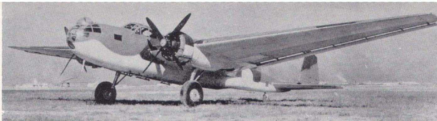
A Ka-15 powered by a pair of Kinsei 2 engines driving fixed pitch four-blade wooden propellers as seen during flight trials.
