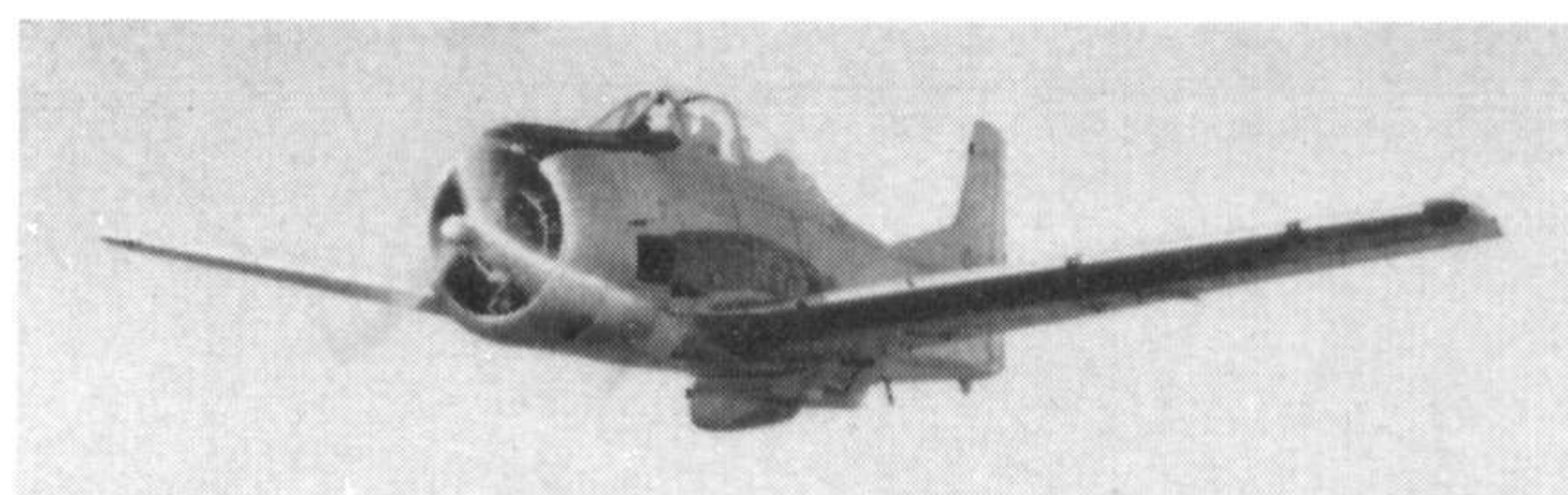
A reconnaissance version of the T-28D carries three cameras in a protruding pack under the belly. (Photo: N.A.A.)
