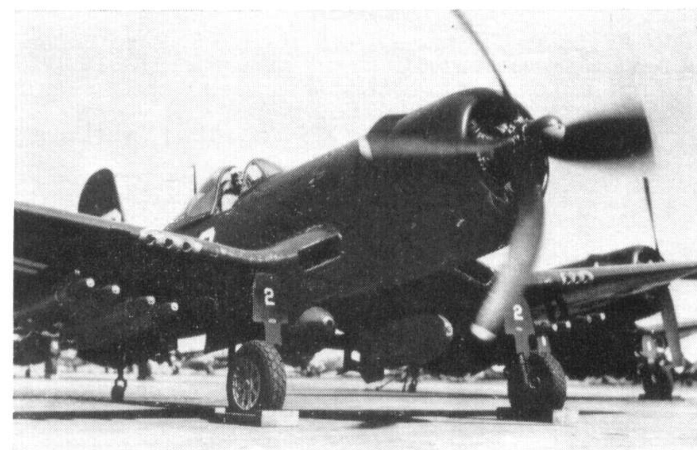
Early rounded windshield on a Korea-based F4U-4.
