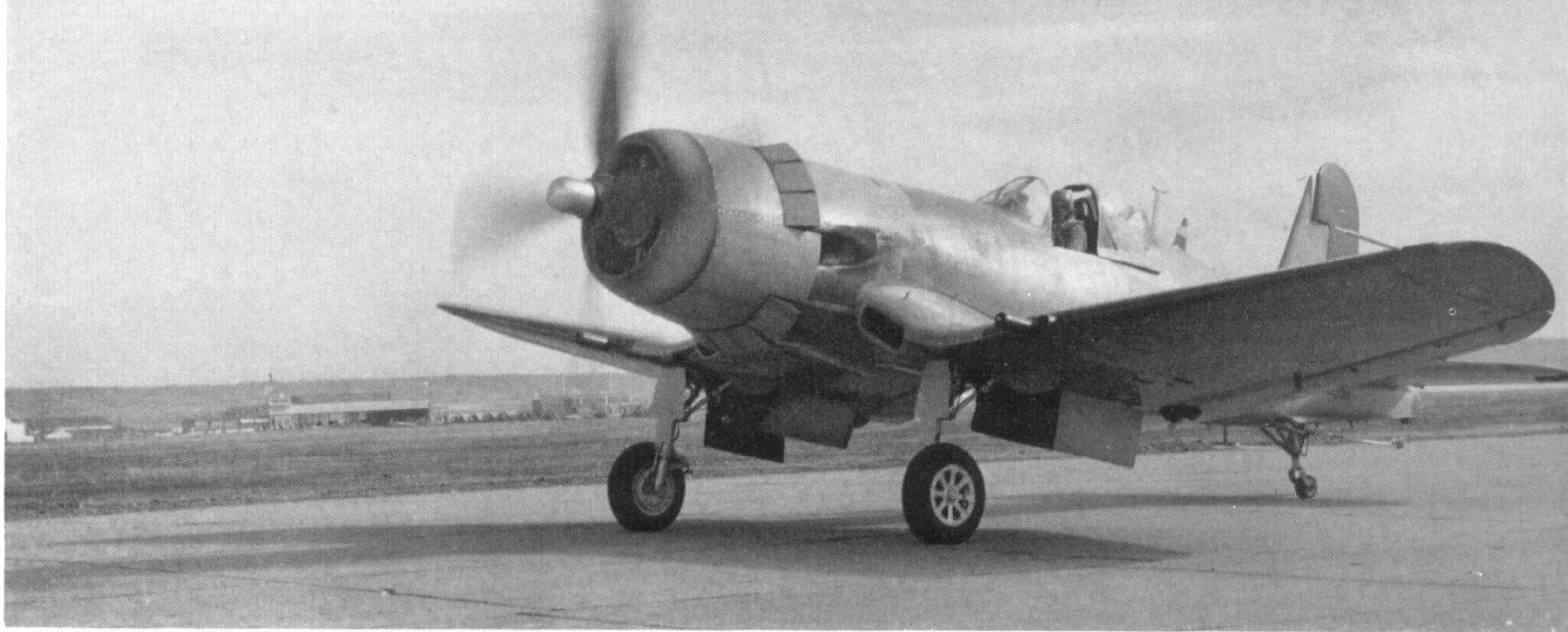
Attractive study of a partially-painted AU-1; only wing outer panels and tail control surfaces are finished in glossy sea blue.
