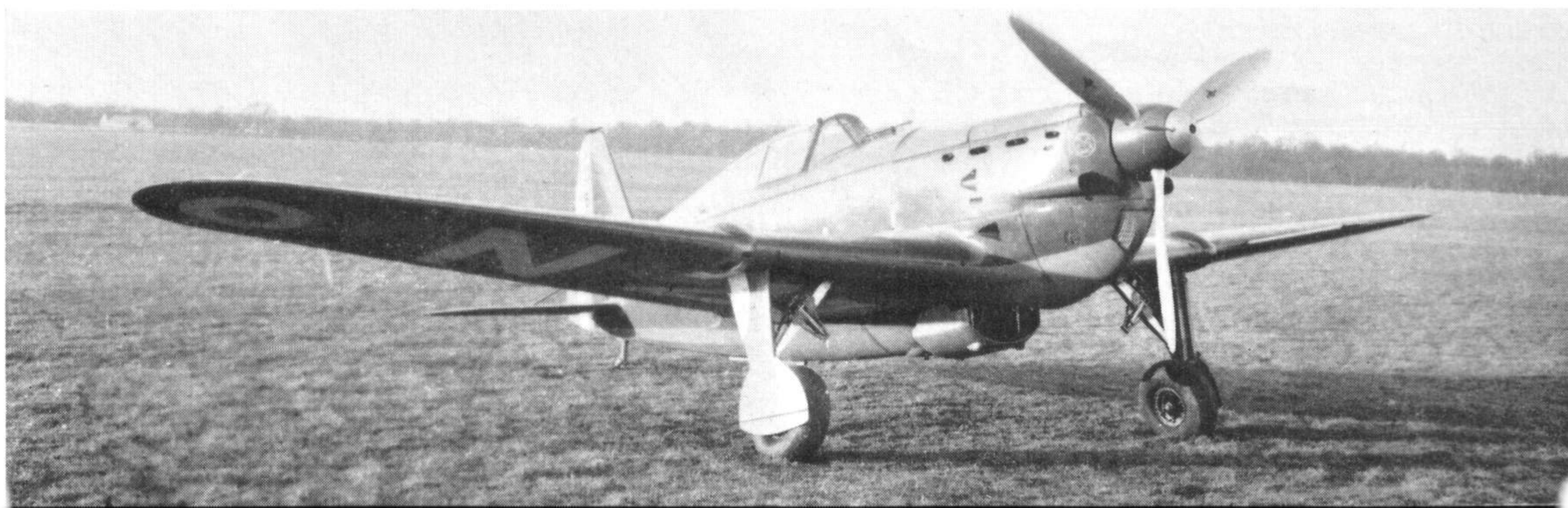
M.S. 405 No. 2; note windmill actuator of airscrew, and long wheel wells.
