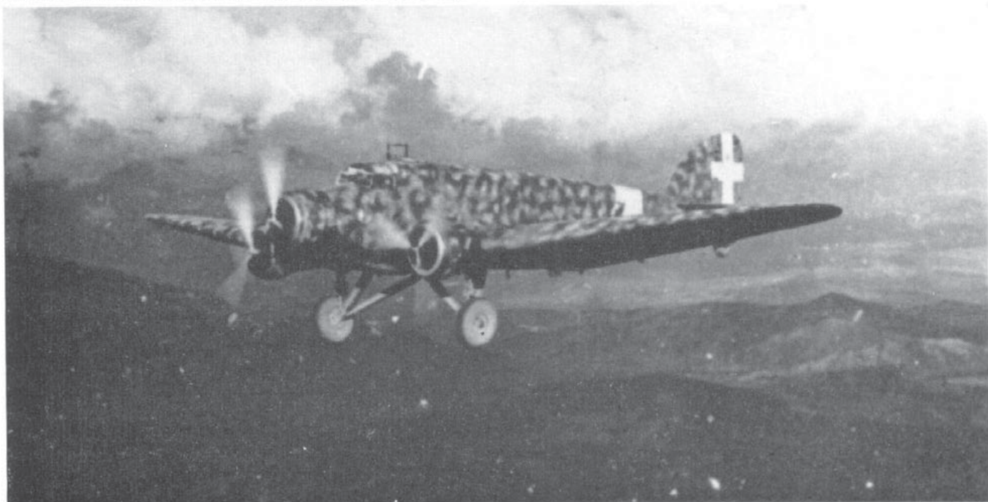
An S.M.81 of the 38 o Stormo flying over Albania during the first phase of the war against Greece. The undercarriage wheel fairings have been removed and the camouflage scheme is noteworthy.
