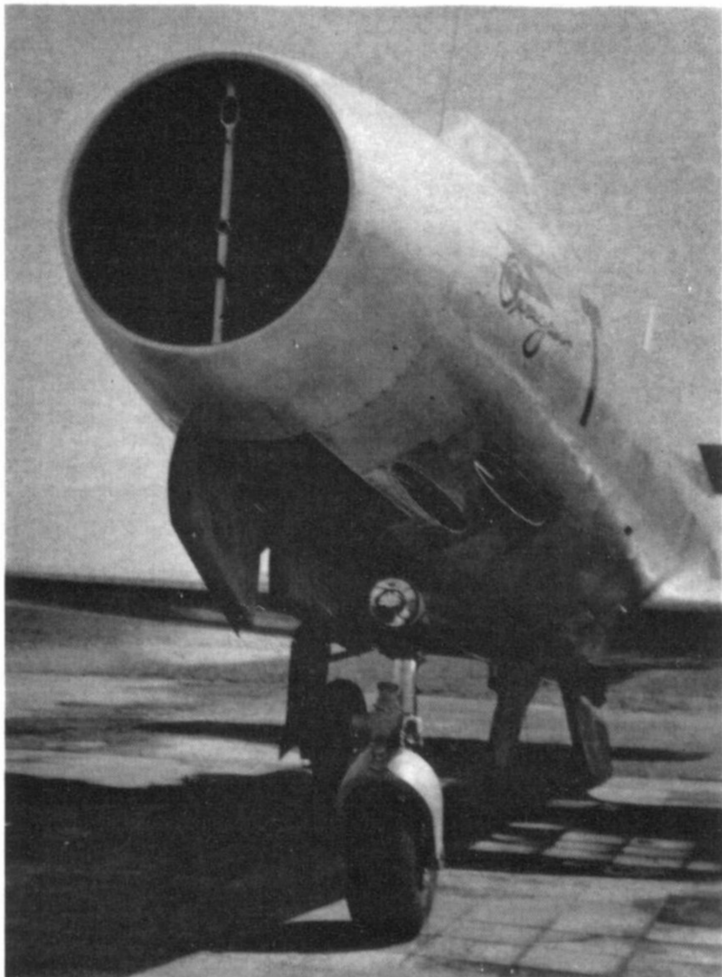
The redesigned two-piece nose wheel door fitted to all production Ouragans from No. 151 onwards.
