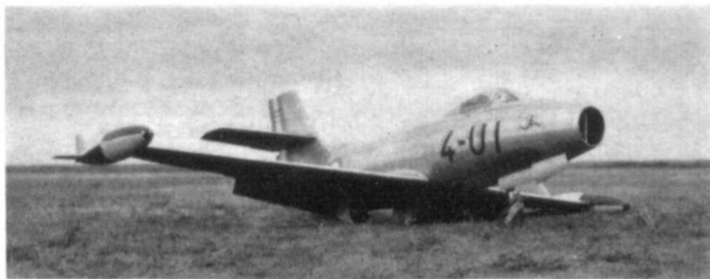
Apparently even the new nose wheel door was not entirely trouble-free. Left: An Ouragan of II/4 with one half closed, one half open. Right: One of III/4's aircraft after an unhappy landing.
