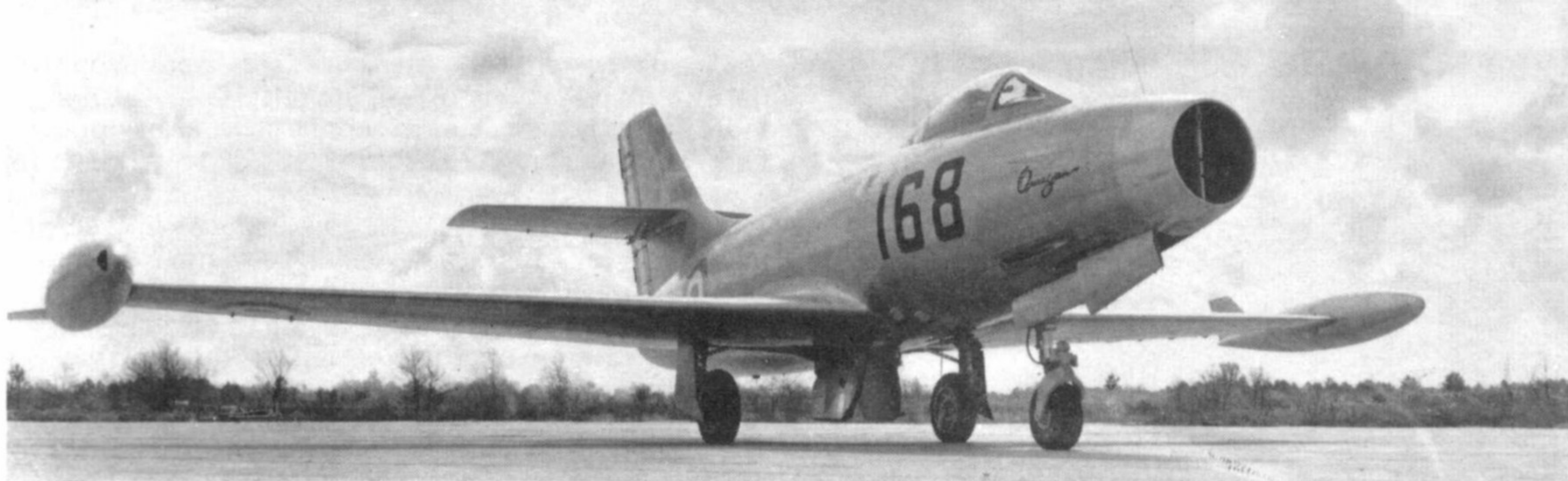
The 68th production Ouragan, displaying the new two-section nose wheel door introduced from the 51st aircraft onwards.
