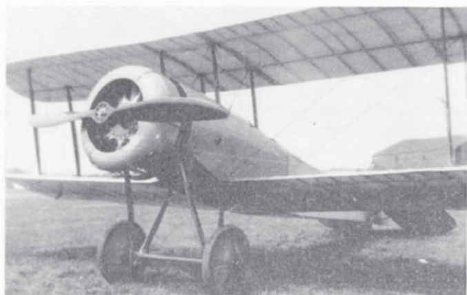
The first Scout after it had been bought by Lord Carbery and fitted with an 80 h.p. Le Rhône engine. With this engine the lower portion of the cowling was extensively cut away.
