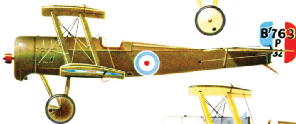
Bristol Scout D, No. B763, as at McCook Field, U.S.A. Note absence of underwing skids, project number under serial on rudder.
