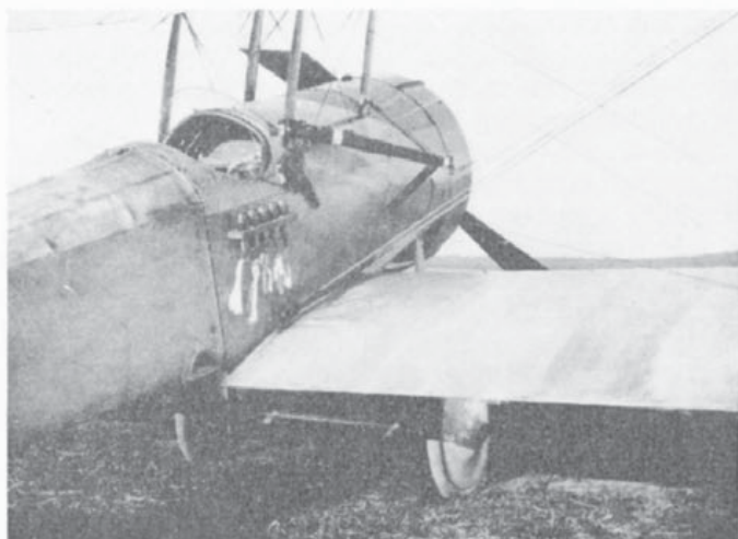
The first Scout after it had been bought by Lord Carbery and fitted with an 80 h.p. Le Rhône engine. With this engine the lower portion of the cowling was extensively cut away.
