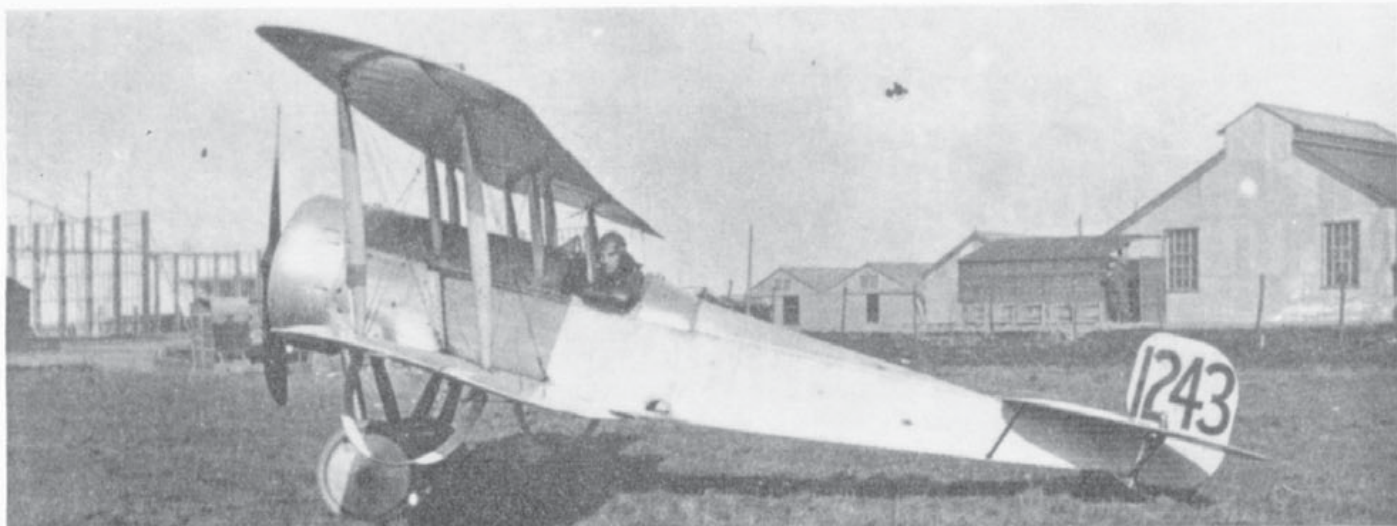
The first production Scout C, No. 1243, at the Isle of Grain. In the cockpit is Flight Sub-Lt. W. G. Moore. The fairings on the wing-tip skids are an unusual refinement.
