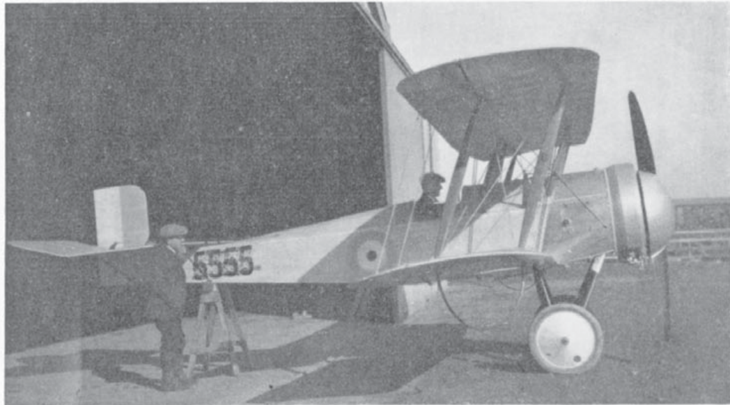
Scout D No. 5555 with 110 h.p. Clerget engine, enlarged cowling and spinner.
