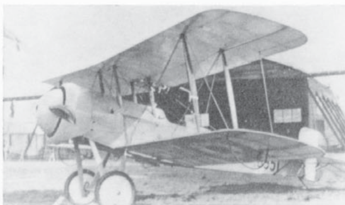
Scout D No. 8951 with spinner on 100 h.p. Monosoupape engine.
