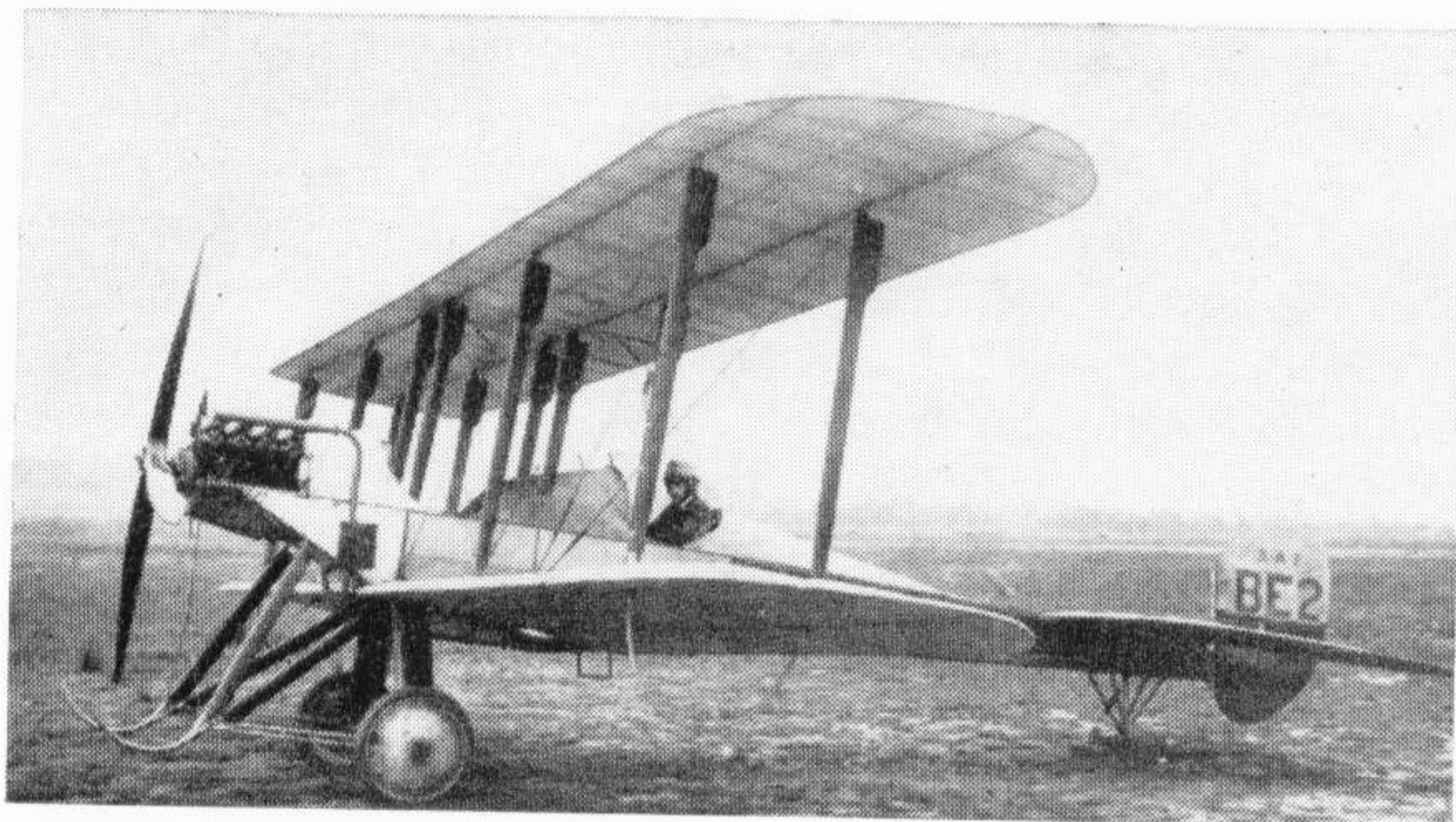
A B.E.2a with an early type of oleo undercarriage and fitted with the fin struts designed by Edward Busk.
