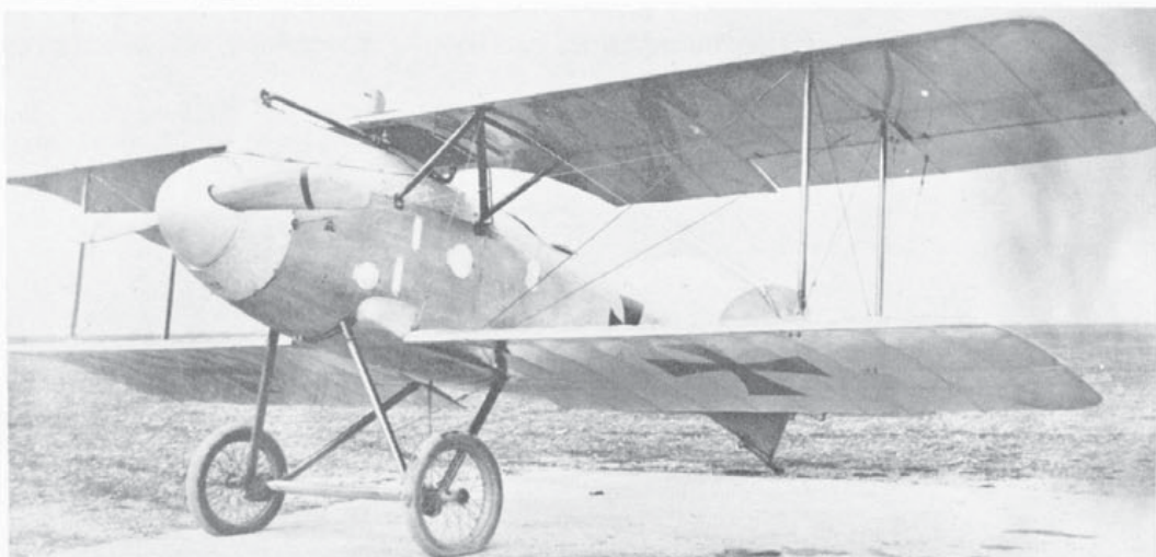
Later type of Albatros D II with flush radiator in centre of upper wing. The racier appearance resulting from the reduced gap is noticeable when compared with the D I. (Photo: Egon Krueger)
