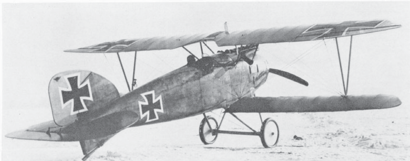
Crisply etched against the winter sky and snow covered airfield the graceful lines of the D III are well shown in this view. This is an early "ex-works" machine with centrally located radiator. (Photo: Egon Krueger)
