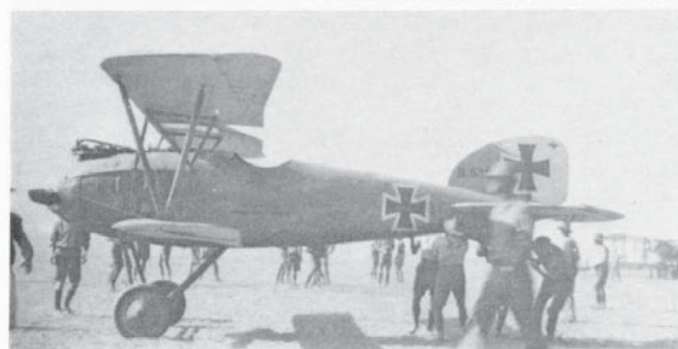
Albatros D III D 630 captured in Palestine. Note gap in centre-section where radiator has been removed. Albatroses in this theatre of war were eventually fitted with twin radiators.
