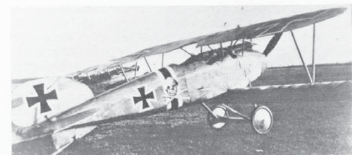
Late model D III fitted with D V type rudder. Insignia appears to be black and white—unit not known.
