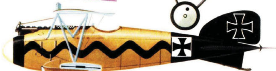
Albatros D III of Jasta 12. Upper surfaces of wings finished in green and mauve camouflage.
