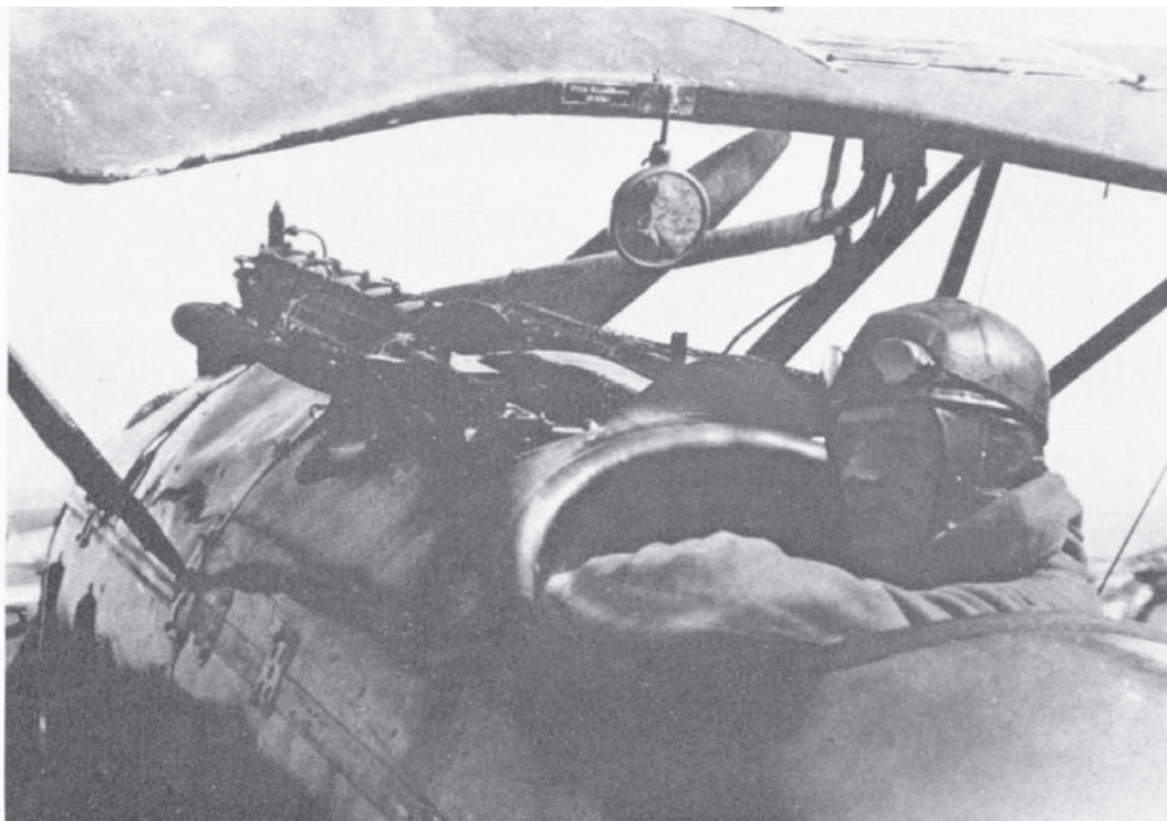
Close up of cockpit and guns also shows rear view mirror and off-set radiator. Vzf.w. Anton Banhofer, Jasta 25 in Macedonia. (Photo: Egon Krueger)
