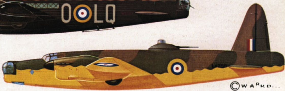
Wellington II, L4250, modified to test 40 mm. Vickers 'S' gun.
