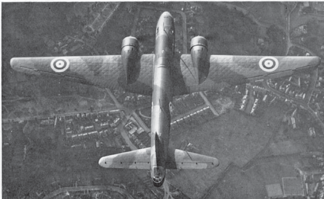
Striking overhead view of a Wellington I on test. Note upper surface structural details.
