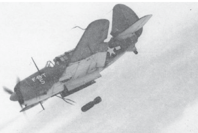
A classic view of an SB2C-1 releasing a 1,000 lb. bomb with the displacement gear. (Photo: U.S.N./National Archives)
