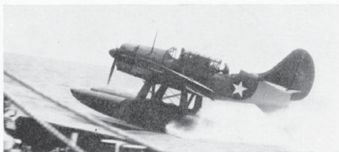
Rough water tests on the XSB2C-2 in Hampton Roads, Virginia were conducted in March 1943 by pilots from NAS Norfolk, Virginia. This shot shows the aircraft immediately after touching down. (Photo: U.S. Navy)
