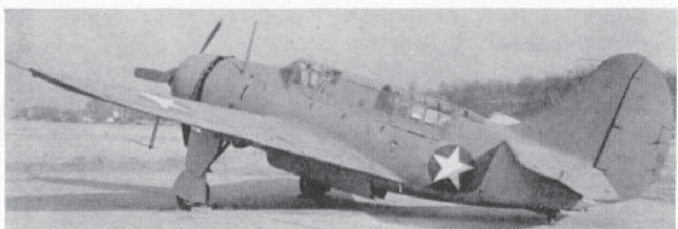
Radio and electrical tests were conducted on 00007 at Anocostia. Photographed on 14th December, 1942, the aircraft is seen here with ASB radar and ABD IFF installed. (Photo: U.S. Navy)
