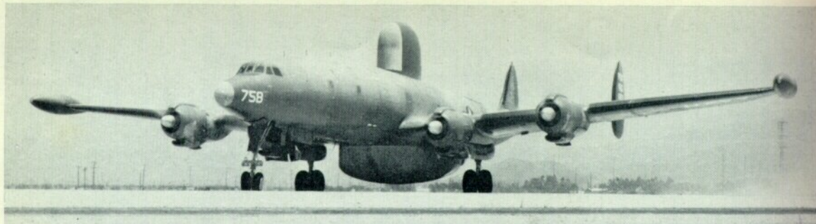
A Pacific Missile Range "Willy Victor" EC-121D takes off from Pt. Mugu on a frequency interference control mission prior to a satellite launching. This study gives an impression of the massive radar bays. (Photo: U.S.N. via Bulban)
