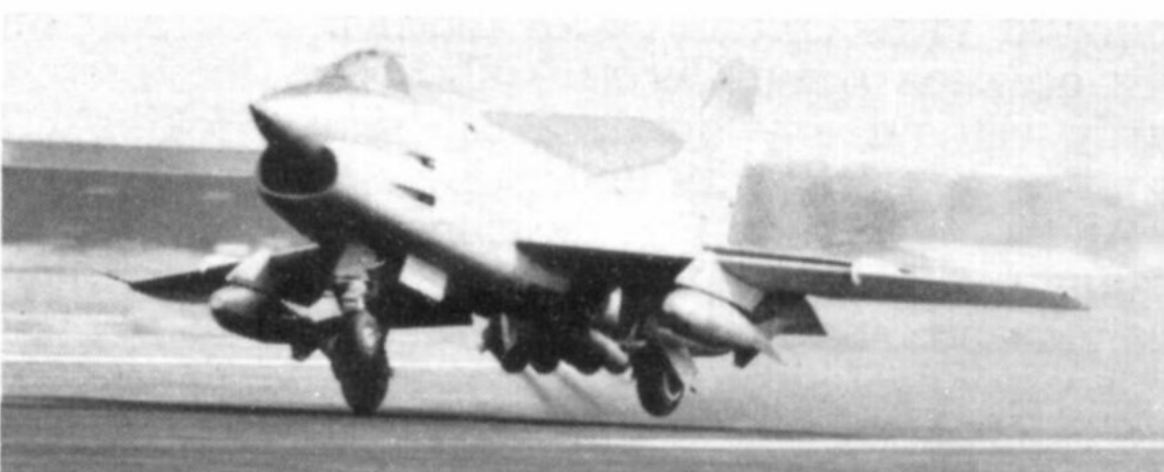
The moment of take-off—with four JATO bottles and two underwing bombs.
