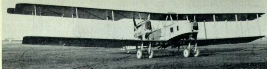
Gotha G.V 904/16 with streamlined engine struts and improved fairing of the lower wing as compared to earlier types.
