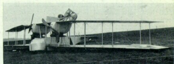
G.I, 14/15 after the fatal crash of Lt. Franz Rosenfeld in October 1915, demonstrating the danger of a high-fuselage nose-over. The accident occurred at Armee Flugpark Falkenhäusen on the Western Front.
