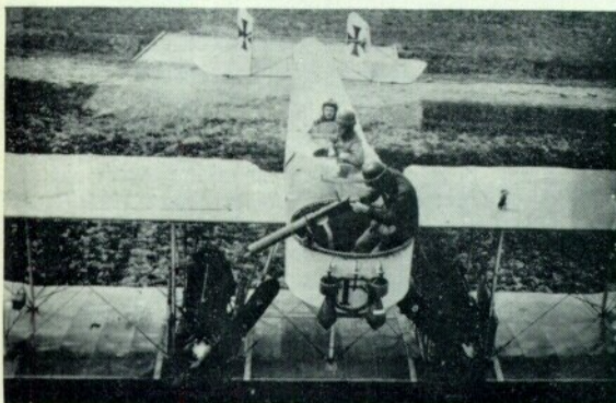
The B.1092/14 at Feld Flieger Abteilung 28 ; the cowlings have been removed for better cooling and new radiators installed. Note the "FU" monogram on the nose. This was the first German twin-engined bomber of the war. (Photo: Egon Krüger)
