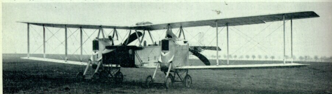
G.II prototype with two-bay wings, four-wheeled undercarriage and simple slab rudder.
