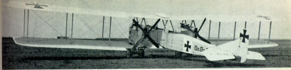
Gotha G.II 204/16 production version here fitted with four-bladed propellers. The paddle-shaped guards on each side of the rear cockpit protected the gunner from debris kicked up by the wheels and flung inboard by the propeller, and also prevented the gunner from accidentally leaning into the aircrew arc. The aircraft is covered with unbleached fabric, note contrast with white field of the crosses.
