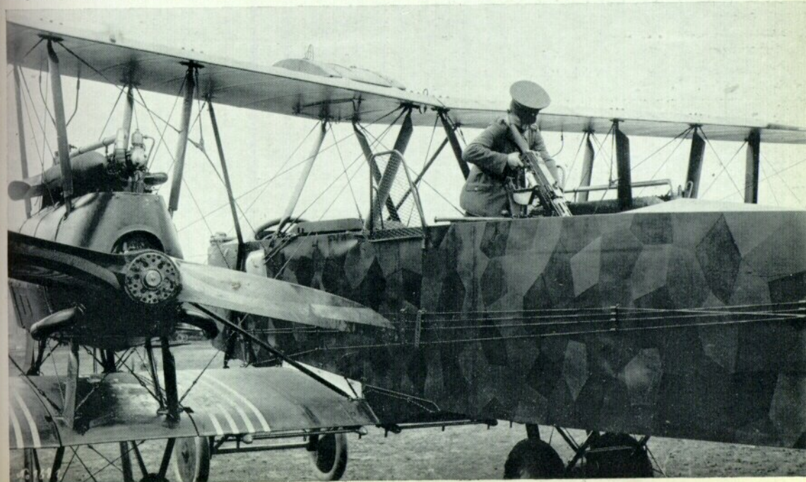
The upper gunner of a G.Va demonstrating the downward-firing capability of his Parabellum machine gun, aiming down through the rear fuselage under-surface cut-out. Note excellent clarity of details of engines and fabric skinning.
