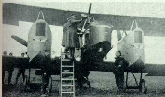
Left: Interested pilots of Jasta 4 examine Gotha G.III 397/16 at Marchais in May 1917. The slim fuselage and Cellon windows on the side of the front cockpit are here evident. Right: G.III 397/16; the passageway on the right side of the fuselage connects the front and rear cockpit; the rear gun is mounted on a lateral slide rail; and mudguards on the wheels prevent stones being thrown into the propeller arc.
