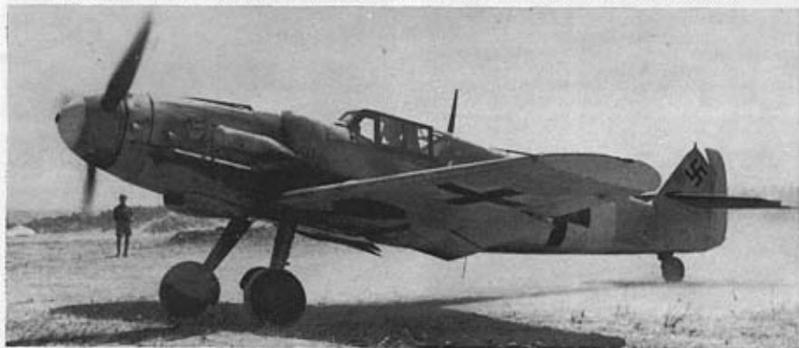
A Bf 109G-1 Trop. of I/JG 51 "Molders" on the South Russian Front. The penetrating dust which characterised Russian airfields in summer forced the installation of sand filters on aircraft in this theatre. Note the Geschwader insignia on the cowl.
