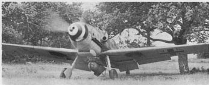
The Gustav runs up in its wooded dispersal point; this sequence was photographed in Russia during the summer battles of 1943. This illustration demonstrates effectively many of the characteristics of the Bf 109G series, including the narrow-track undercarriage, the streamlined air intake on the port side of the cowl, the shallow underwing radiators, and the popular spiral spinner motif, carried both as decoration and as an attempt to put air-gunners off their aim.
