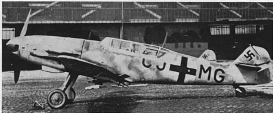
A G-12 two-seat trainer, modified from a G-1 Trop. The instructors' cockpit in the rear had a special bulged canopy to give a degree of forward vision and the two MG 131 weapons in the nose were sometimes retained, as in this case.
