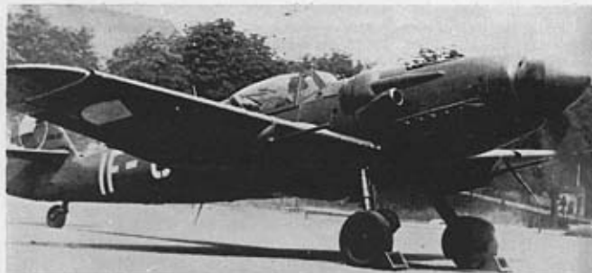
Mezec (Mule) was the name by which the Avia C-210 was known to Czechoslovak pilots; its handling characteristics were said to be vicious. Note that this aircraft has a new blown canopy.
