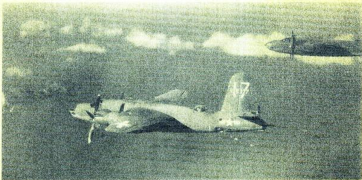
B-26C-25's returning from a mission in Italy. The port engine of the aircraft in the foreground was damaged by German flak at Roccasecca Bridge; on the return flight the crew lightened ship to ease the strain on the starboard engine, jettisoning all movable equipment. As this photograph was taken, a belt of .50 calibre ammunition was dropped from the tunnel gun position.
