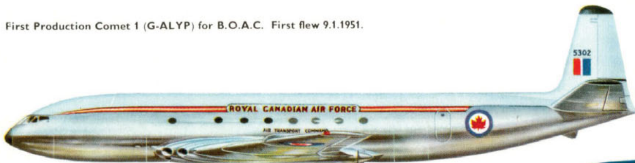
Comet 1A (VC 5302, c/n 06018) second machine for R.C.A.F., shown after introduction of oval cabin windows. Withdrawn from service and stored in 1964.
