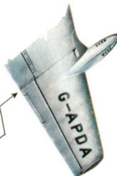
Outer wing and fuel tank of Comet 4. Note greater span
