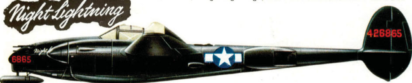
P-38M, 44-26865, "Night Lightning", first P-38M converted from P-38L-5-LO.
