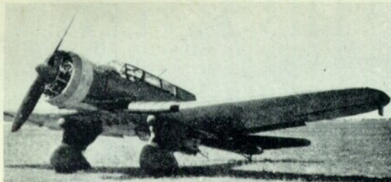
P-23/II Karaś, with the engine mounted in the intermediate position. (Photo: the author)
