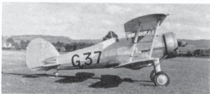
Three interesting comparative views of Gladiators. Top: The Gladiator prototype S.S.37 as it originally emerged from the experimental shops at Glosters. Note open cockpit, drum-fed Lewis guns under the lower wings, narrow-chord engine cowling and unfaired wheel discs. Centre: The same aircraft after modification to full production standard with Service serial, enclosed cockpit, Browning underwing guns, Mercury VIII engine and faired wheel discs. The spatted tailwheel has however been retained. Bottom: The second production Gladiator I, K6130, with unspatted tailwheel and minor alterations to the radio aerial. (Photos: Upper, Flight Neg. No. 10763s; Centre, Gloster Aircraft Co. Neg. No. G105; Lower, Ministry of Defence Neg. No. 8995D).
