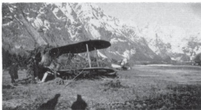
A No. 263 (Fighter) Squadron Gladiator at Aandalsnes in 1940. This photo, which also shows a Fleet Air Arm Skua in the background, gives some indication of the rugged Norwegian terrain, while the care taken to disperse and camouflage the aircraft suggests an acute awareness of the proximity of enemy forces. Also of interest is the absence of wheel discs, the removal of which was found to be necessary owing to the pervading mud and moisture freezing and locking the wheels; this expedient was a relic of No. 263's preparations for action in Finland, and was adopted throughout the Norwegian campaign. (Photo: Air Commodore Whitney W. Straight)
