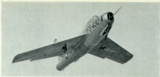
The prototype after being rebuilt with the British Sapphire engine. (Photo: Republic)
