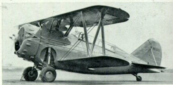
Above: Al Williams' NR1050 Gulfhawk II; highly polished chrome struts combined with brilliant orange finish and blue and white trim to produce an extremely colourful aeroplane. In contrast to other F3F types, the span was 28 ft. 6 in., and the machine had improved spin characteristics. (Photo: Besecker Collection). Below: NC1051 Gulfhawk III is less well known than the single-seater; this G-32 design had split flaps on upper wing. (Photo: Grumman)
