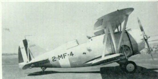
F3F-1 (0256) as leader of second section of VMF-2. Note Marine insignia under cockpit and .50 calibre blast tube visible over cowling.
