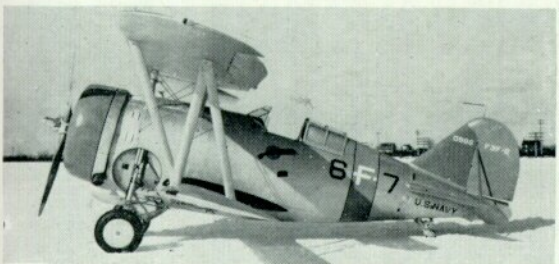
F3F-2 (0986) factory fresh at Bethpage, Long Island, before delivery to VF-5. Note louvre above leading edge of stabiliser designed to reduce CO content in cockpit.
