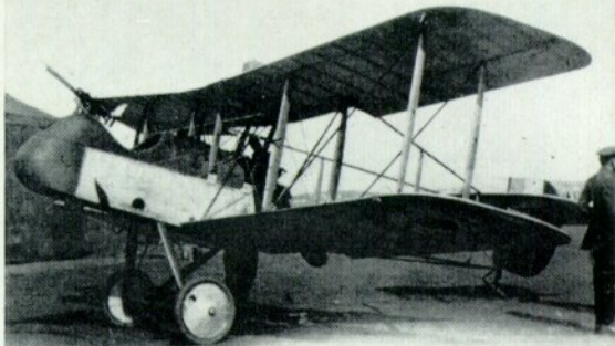
On this D.H.2 the windscreen was mounted on the rear of the Lewis gun, which is seen partly elevated.
