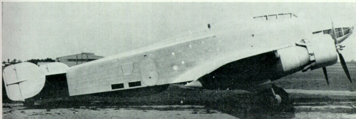
One of four S.M.79Bs acquired for the Iraqi Air Force in 1938; powered by Fiat A.80 engines, these machines were eventually destroyed during the anti-British rising in 1941. (Photo: R. Ward Collection)
