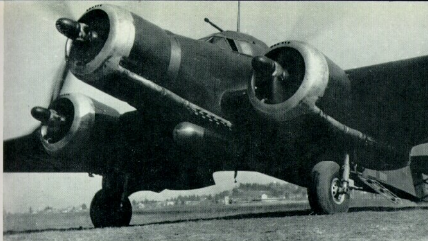
The single off-set torpedo installation more usually carried by the Aerosiluranti, seen here on an S.M.79III. Note absence of ventral gondola, lengthened airscrew hubs, extended exhaust manifolds, and the forward-firing 20-mm. cannon above the cockpit. Produced in small numbers only, the S.M.79III was operated in the Mediterranean by Capt. Faggioni's torpedo-bombing Group. (Photo: via the author)
