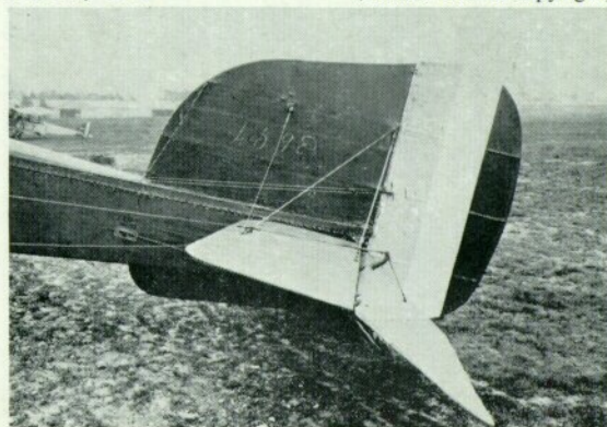
A3406 fitted with the enlarged fin and balanced rudder designed for the R.E.8 but almost indistinguishable from the corresponding surfaces designed for the R.E.9 and R.T.1.
