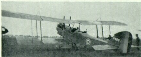
A3406 fitted with the enlarged fin and balanced rudder designed for the R.E.8 but almost indistinguishable from the corresponding surfaces designed for the R.E.9 and R.T.1.
