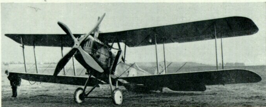
R.E.9 A3561 with Sunbeam Maori engine, 23rd September 1918.
