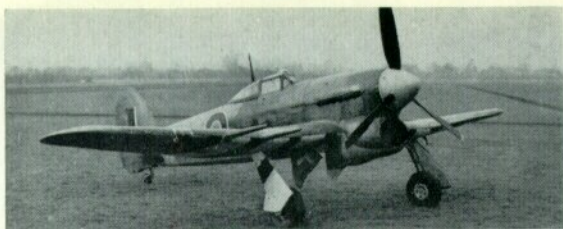
Cleaning up the Typhoon. A programme was initiated in 1942 to increase the performance by attention to detail; pictures of R8809 show the change in hood shape, elimination of external rear view mirror, adoption of whip aerial, fairing of cannon barrels and addition of exhaust manifold plinth.
