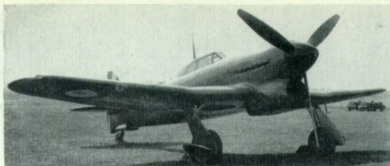
Two early photos of the second Typhoon prototype, P5216. That on the left, taken at Boscombe Down, shows the 12-gun wing to advantage as well as the hinged door flaps attached to the leg fairings. Note also the tailwheel doors. Right: A later photo taken at Langley after the tailwheel doors had been removed.
