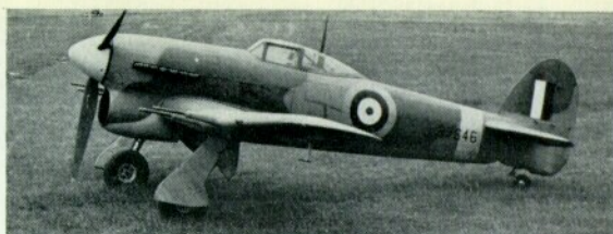
First Gloster-built Typhoon to be fitted with rear-vision hood. The photo, taken during assembly at Hucclecote, also shows the engine and radiator installation, whereas the other picture was taken during evaluation by Hawker pilots at Langley.
