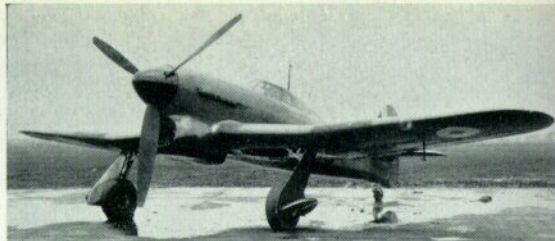
Two early photos of the second Typhoon prototype, P5216. That on the left, taken at Boscombe Down, shows the 12-gun wing to advantage as well as the hinged door flaps attached to the leg fairings. Note also the tailwheel doors. Right: A later photo taken at Langley after the tailwheel doors had been removed.
