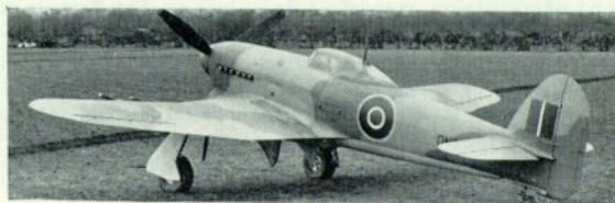
Two views of one of the tropical Typhoons. Just visible is the ventral air exit fairing between the central wheel doors. Colour scheme was sand and dark green upper surfaces and pale blue undersurfaces. Two other Typhoons, R8925 and R8889, were also equipped for tropical trials and all were shipped to Khartoum early in 1943.
