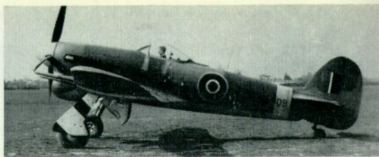
Cleaning up the Typhoon. A programme was initiated in 1942 to increase the performance by attention to detail; pictures of R8809 show the change in hood shape, elimination of external rear view mirror, adoption of whip aerial, fairing of cannon barrels and addition of exhaust manifold plinth.
