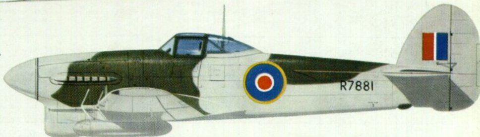
Sole Typhoon N.F.IB, R7881, with A.I. Mk. IV radar, Boscombe Down and F.I.U., Ford, 1942-43.
