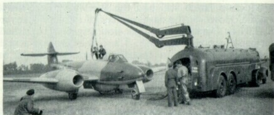
In the field with the Meteor 4. Above: high-speed refuelling of a Norwegian Mk. 4. Below: armourers change the four 20-mm. cannon. (Photos: Ministry of Defence)
