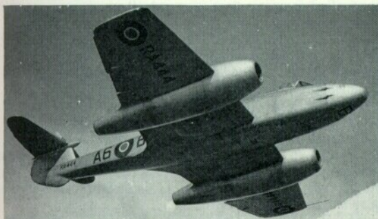
Side, rear and underside flying view of a typical Meteor F. Mk 4 powered by Rolls-Royce Derwent 5 turbo-jets. E.E.592 was a type G.41F Gloster-built aircraft. (Photos: Ministry of Defence)
