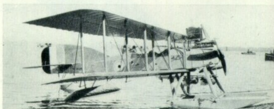
Left: The installation of the 240-h.p. Sunbeam Gurkha in No. 8014 did not differ externally from that of the 225-h.p. engine. The aircraft is seen at Grain on 9th December 1916, fitted with the underslung bomb rail with racks for four bombs. (Photo: Imperial War Museum MH2869.) Right: The Dover-type Renault installation with central elevated radiator, here exemplified on Short 184 N1616 built by Saunders.
