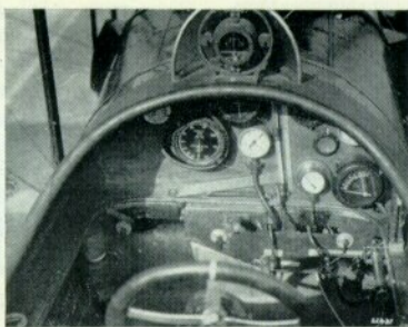
Left: This view of the cockpits of N1086 suggests that one reason for reverting to the single central radiator for the Renault engine may have been to improve the pilot's view for landing. Middle: There was no truly standard cockpit layout for Short 184s, as these illustrations show. This is the dashboard of 8076, the Short-built Maori-powered 184 that appears in other illustrations. Right: The pilot's dashboard on N1081, Short-built Improved 184 with 240-h.p. Renault engine.
