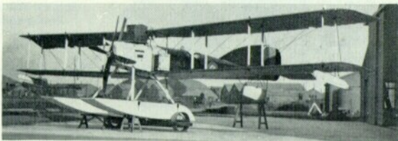
This Type D is No. 9048, built by Robey and powered by a 240-h.p. Sunbeam Gurkha driving a four-blade airscrew. Like No. 8359, it had a stack-type exhaust pipe.
