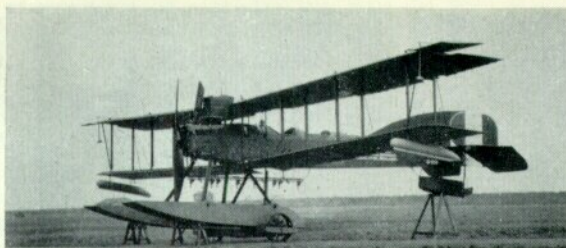
No. 8076 at the Isle of Grain, fitted with Martin stabilisers on the upper wings, 5th November 1917.
