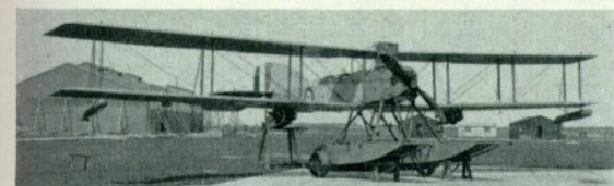
No. 8052 with two 65-lb. bombs under each lower wing. This was an early attempt to fit bomb racks to the Short 184 but was abandoned in favour of the under-fuselage bomb rail. This Short still had arched float cross-bars when this photograph was made.
