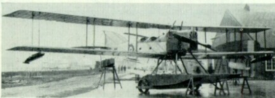
This Type D is No. 9048, built by Robey and powered by a 240-h.p. Sunbeam Gurkha driving a four-blade airscrew. Like No. 8359, it had a stack-type exhaust pipe.
