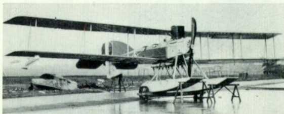
Left: The installation of the 240-h.p. Sunbeam Gurkha in No. 8014 did not differ externally from that of the 225-h.p. engine. The aircraft is seen at Grain on 9th December 1916, fitted with the underslung bomb rail with racks for four bombs. (Photo: Imperial War Museum MH2869.) Right: The Dover-type Renault installation with central elevated radiator, here exemplified on Short 184 N1616 built by Saunders.
