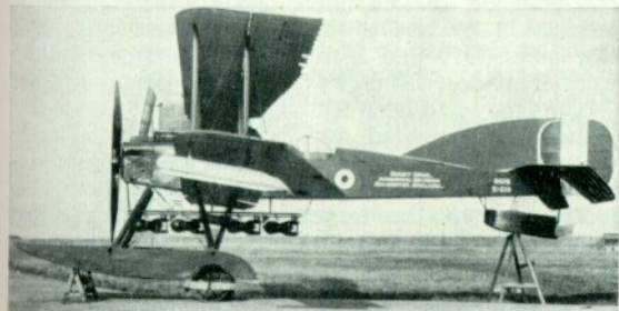
No. 8076 at the Isle of Grain with Whitehouse gun mounting on the rear cockpit and four 100-lb. bombs. This aircraft had a 260-h.p. Maori I or II driving a two-blade airscrew.
