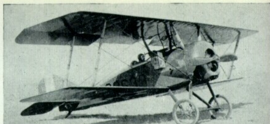
Left: S-4C formerly owned by Jack Walton of Tampa, Fla., photographed in 1937. This is probably the prototype S-4 with S-4C wings and Le Rhône engine; the fuselage is longer than the standard S-4C. (Photo: Jack Walton). Right: The first Tommy with Le Rhône engine, S-4C 38633, photographed at Taliaferro Field, Hicks, Texas. Note field modification of box for expended cartridge cases, and rudder from different aircraft, 38651. (Photo: Air Force Museum)
