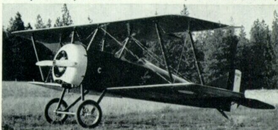
No. 38898 (now re-named Carlson S-4C) during final stages of rebuilding by Ed Carlson; rigging not complete. Powered by 120-h.p. Ken Royce radial.
