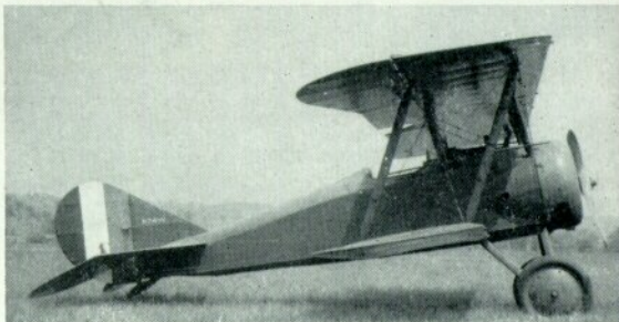
S-4B No. 153, the only surviving example, owned by the late D. B. Woodward and now on loan to the U.S.A.F. museum, Dayton, Ohio. A machine gun has been added, and original 100 h.p. Gnome has been replaced by 80 h.p. Le Rhône.
