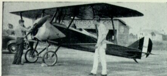
Left: S-4C formerly owned by Jack Walton of Tampa, Fla., photographed in 1937. This is probably the prototype S-4 with S-4C wings and Le Rhône engine; the fuselage is longer than the standard S-4C. (Photo: Jack Walton). Right: The first Tommy with Le Rhône engine, S-4C 38633, photographed at Taliaferro Field, Hicks, Texas. Note field modification of box for expended cartridge cases, and rudder from different aircraft, 38651. (Photo: Air Force Museum)
