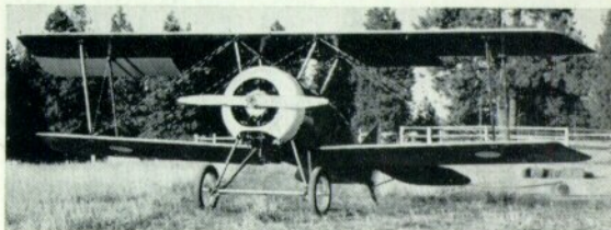
No. 38898 (now re-named Carlson S-4C) during final stages of rebuilding by Ed Carlson; rigging not complete. Powered by 120-h.p. Ken Royce radial.
