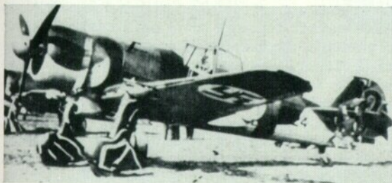
VL-built Fokker D.XXI, FR-124, powered by the Twin Wasp Junior engine, shows off one variation of the undercarriage decoration employed by some Finnish fighter units in 1941.
