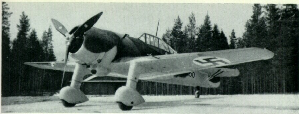
This Wasp D.XXI, probably FR-150, displays the small reproduction of the Finnish swastika insignia carried on each propeller blade by VL-built machines.
