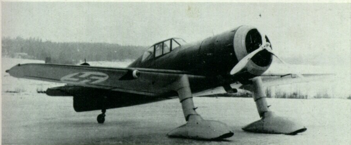
Above: Another Mercury-powered D.XXI of the initial Finnish batch. Note wingtip light and pitot head. Below: Mercury-powered Finnish D.XXI with "snow-shoe" (faired ski) undercarriage.
