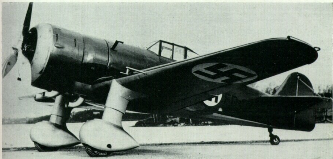
Above: Another Mercury-powered D.XXI of the initial Finnish batch. Note wingtip light and pitot head. Below: Mercury-powered Finnish D.XXI with "snow-shoe" (faired ski) undercarriage.
