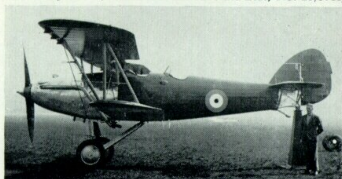
Left: Hart Trainer, K3153, in the markings of No. 10 F.T.S.; note the blind flying hood over rear cockpit. (Photo: K. J. Blackston.) Right: Late-series Hart Trainer K4751 with yellow-painted fabric-covered surfaces. (Photo: Hawker Aircraft Ltd., No. 25/59H)
