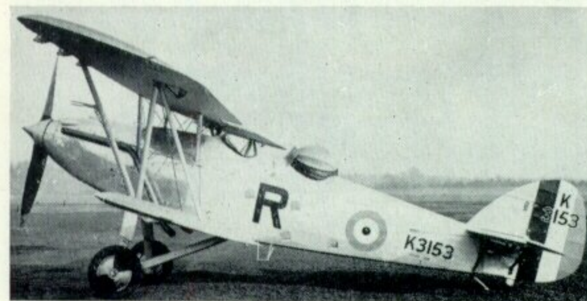
Left: Hart Trainer, K3153, in the markings of No. 10 F.T.S.; note the blind flying hood over rear cockpit. (Photo: K. J. Blackston.) Right: Late-series Hart Trainer K4751 with yellow-painted fabric-covered surfaces. (Photo: Hawker Aircraft Ltd., No. 25/59H)
