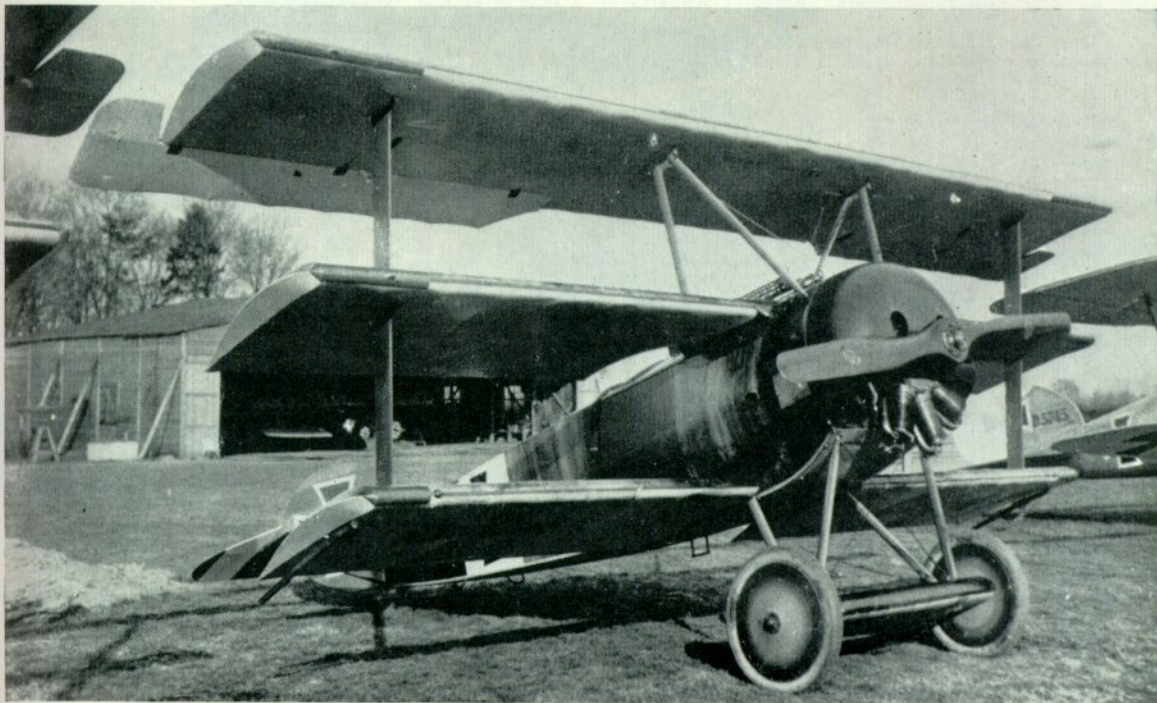
Standard production Fok. Dr.I with late-type ailerons and 110-h.p. Oberursel UR.II engine.
