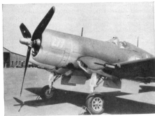
The F4U-1C, with four .50 mm. M-2 cannons. (Photo: Vought)
