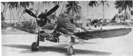
The famous "Ole" 122, an F4U-1A of VMF-111 "Devil Dogs". This aircraft completed 100 dive-bombing missions against Japanese positions in the Marshall Islands, and had an official citation varnished into her cockpit. Note the 300-lb. bomb on a Brewster centre-line rack and the 100 mission markers under the cockpit. (Photo: Vought)
