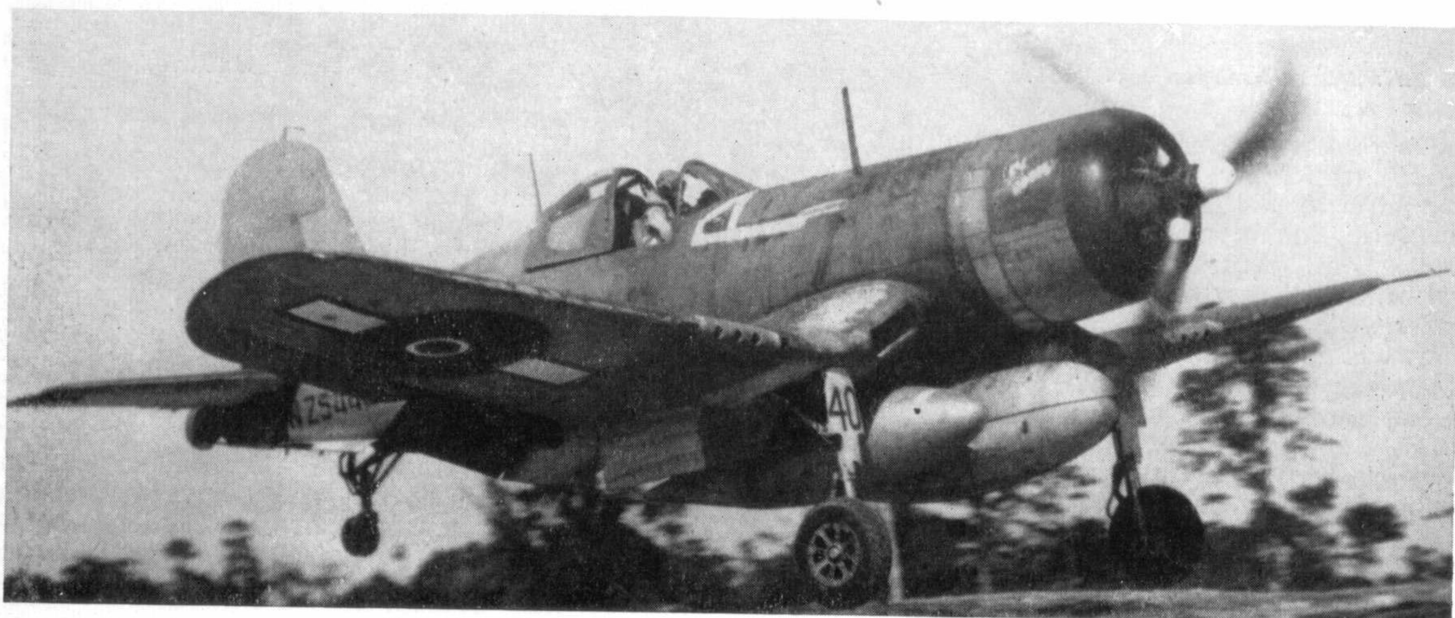
New Zealand Corsair with centre-line and wing-root fuel tanks.
