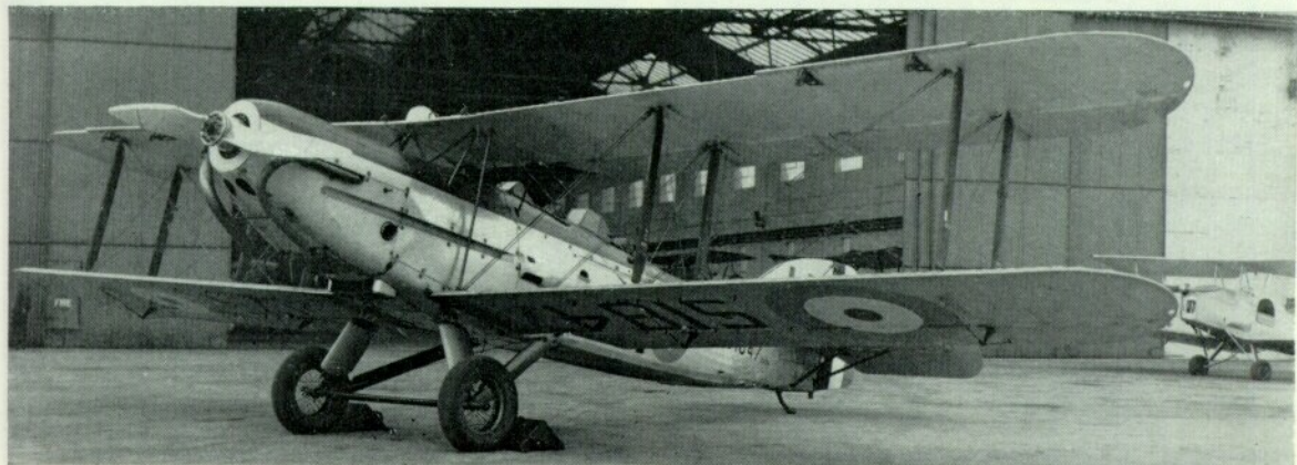
With guns omitted, S1847 was converted from IIIF Mk. III standard to IIIF (DC) standard. Seen here at Martlesham Heath, this dual-control trainer was evaluated for the Fleet Air Arm—evidenced by the jury strut necessary for wing folding. Significance of the “H” on the fin is not known but may be a relic of a previous unit. Below: S1847, frontal view.
