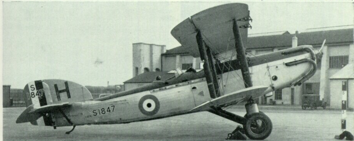
With guns omitted, S1847 was converted from IIIF Mk. III standard to IIIF (DC) standard. Seen here at Martlesham Heath, this dual-control trainer was evaluated for the Fleet Air Arm—evidenced by the jury strut necessary for wing folding. Significance of the “H” on the fin is not known but may be a relic of a previous unit. Below: S1847, frontal view.
