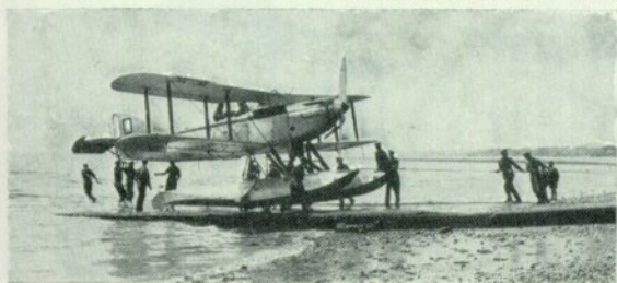
S1317, a IIIF Mk. III, was one of several examples used for catapult trials with the Catapult Flight at Leuchars. (Photo: Ministry of Defence)
