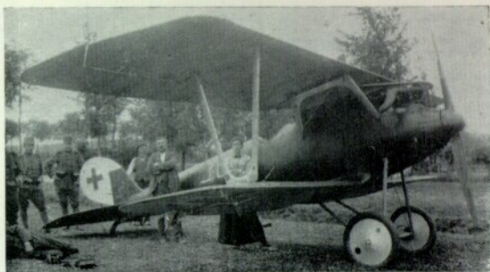
Rare shot of one of the 1918 batch of Pfalz D IIIa's—1306/18 with dark-painted (? black) fuselage and lonzenge-painted fabric underneath wings. (Photo: P. M. Grosz)
