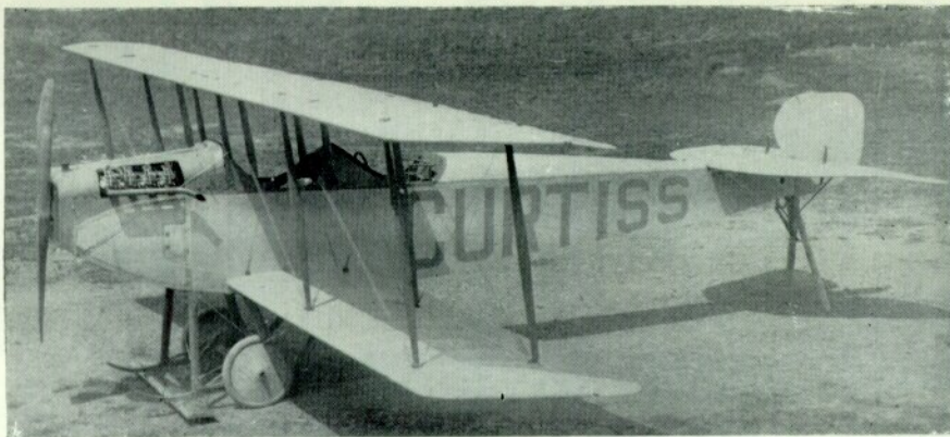
The Curtiss Model "J" in completed form. Its initial flights had been made without fabric covering on the fuselage.
