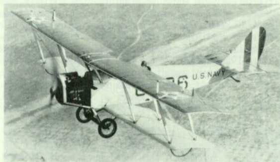
Left: U.S. Navy JN-4H in postwar colouring with reduced-size wing markings. Note that this machine is being flown without the side engine cowling. Right: Early JN-6HB with the larger Curtiss Model “R” vertical tail. Note bomb racks mounted aft of undercarriage.
