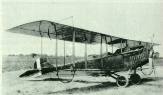
Left: U.S. Navy JN-4H in postwar colouring with reduced-size wing markings. Note that this machine is being flown without the side engine cowling. Right: Early JN-6HB with the larger Curtiss Model “R” vertical tail. Note bomb racks mounted aft of undercarriage.
