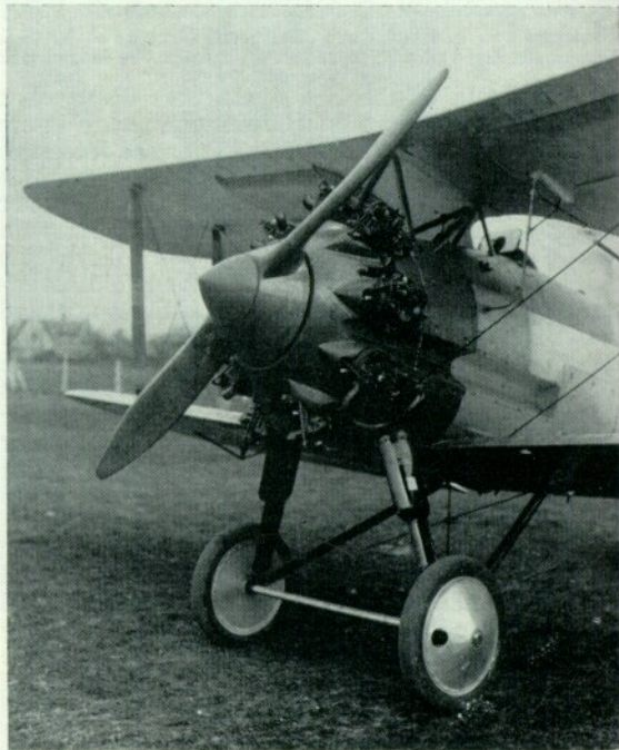
The Gamecock prototype and company demonstrator. Differences lay in the exhaust manifold and spinner. The close-up view (above) shows the demonstrator G-EBNT. Photos taken in March 1926.
