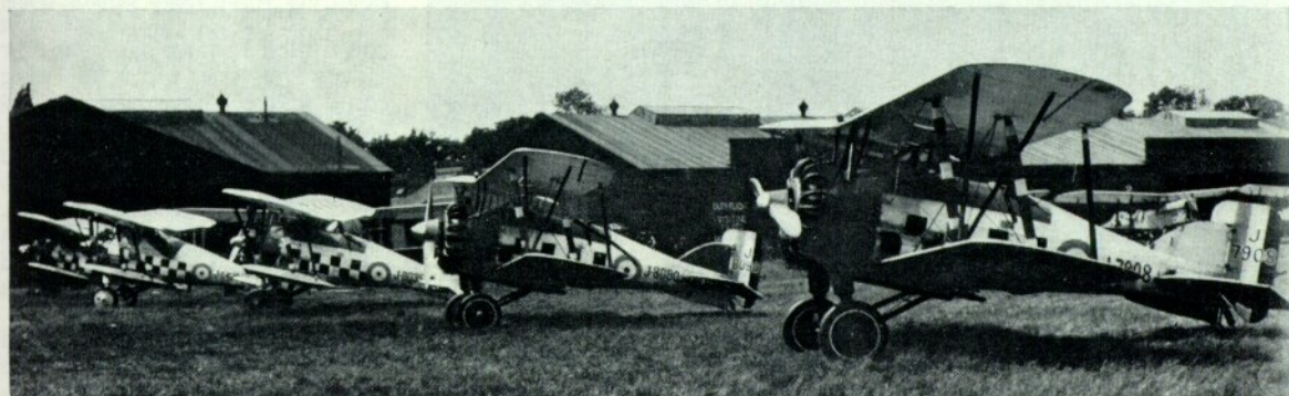
Gamecocks of No. 43 (Fighter) Squadron at the Birmingham Air Pageant of June 1928. Note additional interplane struts and also Flight Commander's pennants, coloured wheel discs and fins.
