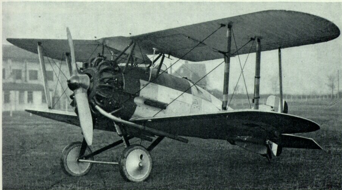
Gamecocks of No. 43 (Fighter) Squadron at the Birmingham Air Pageant of June 1928. Note additional interplane struts and also Flight Commander's pennants, coloured wheel discs and fins.
