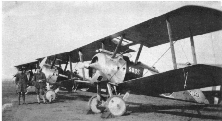
Standard Le Rhône Camels equipped for night flying with flare brackets and navigation lights. These aircraft are said to have belonged to No. 44 (Home Defence) Squadron, but it is equally possible that they may have belonged to No. 78. (Photo: K. M. Molson)
