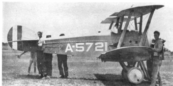
F.1 Camel of the U.S. Navy with hydrovane in front of landing wheels and Grain flotation gear under lower longevanes. (Photo: Fred C. Dickey, Jr.)
