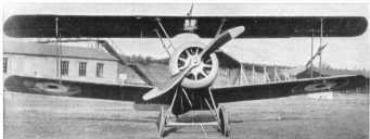
The Sopwith TF.1, with two downward-firing Lewis guns between the undercarriage legs and a third Lewis gun above the centre section. The underside of the fuselage was armoured back to the rear of the cockpit.
