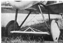
Left: The 9-inch (chord) hydrovane fitted in front of the undercarriage of B3878, August 1918. Right: The tail-skid of B3878 was fitted with a small hydrovane. This was intended to prevent the aircraft from nosing over after alighting.
