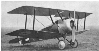
This may have been the F.1/2. It had the one-piece upper wing, original ailerons and the same disposition of the metal cowl panels as the F.1, but a central cut-out was provided in the upper wing and there was a windscreen.
