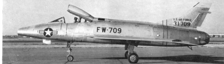
The first F-100C-1 with original short fin and rudder.
