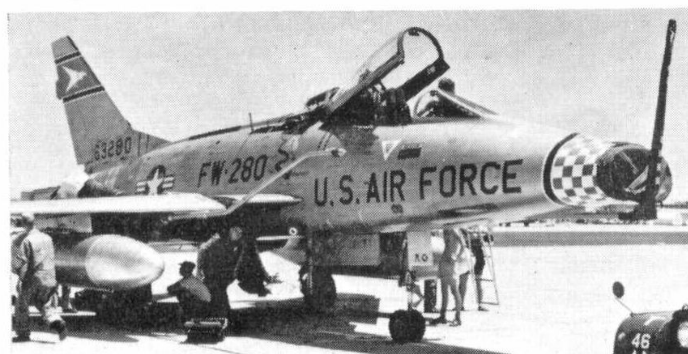
Below: FW-280 displays flight refuelling probe. Note various markings on nosewheel doors. (Photos: via Richard Ward)
