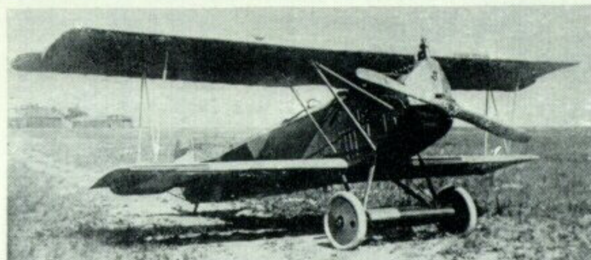
Fokker D VII built by Allgemeine Ungarische Maschinen Fabrik A.G. (M.A.G.) of Budapest. It was fitted with 210-h.p. Austro Daimler engine and radiator similar to the type used on Austrian Berg D I fighter. (Photo: Pavel Vancura)
