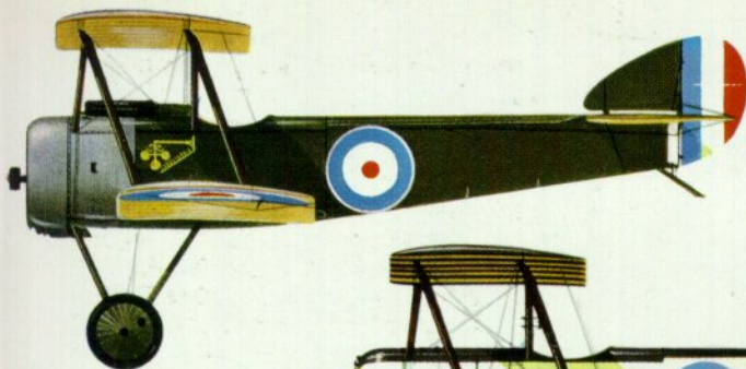
Sopwith Pup, 100 h.p. Gnome Monosoupape, Goşport School of Special Flying, 1917. Flown by Captain Foote. →
