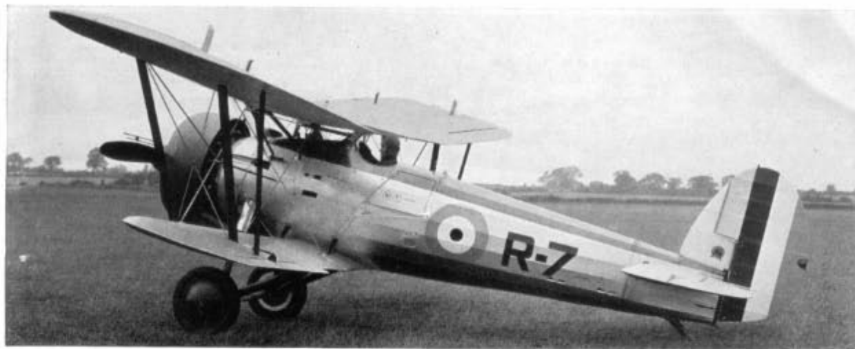
The second Bulldog IIIA, R-7, c/n 7745, private venture aircraft. Registered G-ABZW on 3rd October 1932 but never carried marks. Narrow-chord ailerons on upper and lower wings as standardised on Marks IV and IVA.
