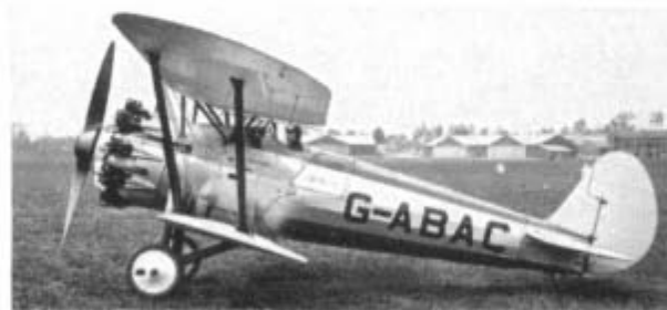
Left: Bulldog II, c/n 7399, SBAC number R.I. Test bed for Mercury III engine fitted with four-blade propeller. Right: R.I with Gnome-Rhône Jupiter VI engine. Registered G-ABAC on 30th May 1930 and destroyed on 4th June.
