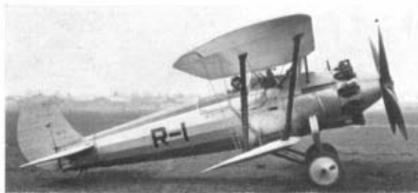
Left: Bulldog II, c/n 7399, SBAC number R.I. Test bed for Mercury III engine fitted with four-blade propeller. Right: R.I with Gnome-Rhône Jupiter VI engine. Registered G-ABAC on 30th May 1930 and destroyed on 4th June.
