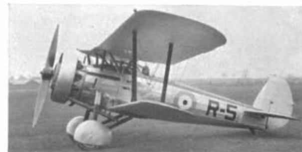
Above: Bulldog IIIA, R-5, c/n 7560, prototype. Built as private venture and first flown 17th September 1931. Mercury IVA engine and spats. Below, top: R-5 with Mercury IVS.2 engine, June 1932. Bottom: R-5 without cowling and spats and with Mercury IVS engine.
