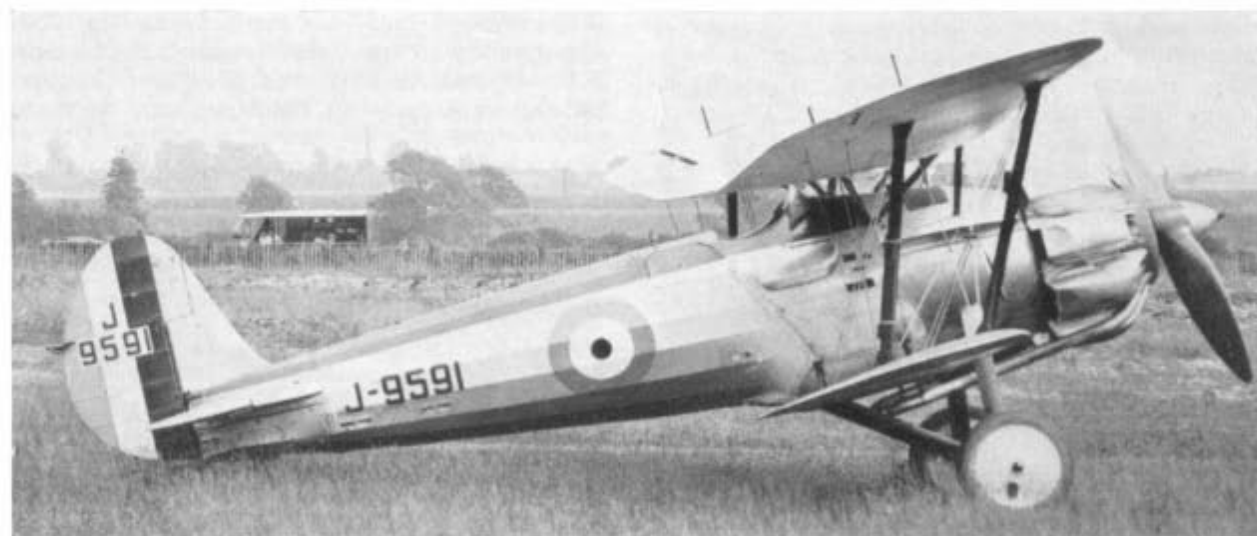
Bulldog II, J9591, c/n 7397, as used for flight testing the geared Mercury IV with cylinder-head helmets. Registered G-AATR on 13th January 1930 but reverted to original serial in January 1931 for tests with Mercury IV/A. Entered R.A.F. service in September 1931 with normal Jupiter VIIIF as on standard R.A.F. Bulldogs.
