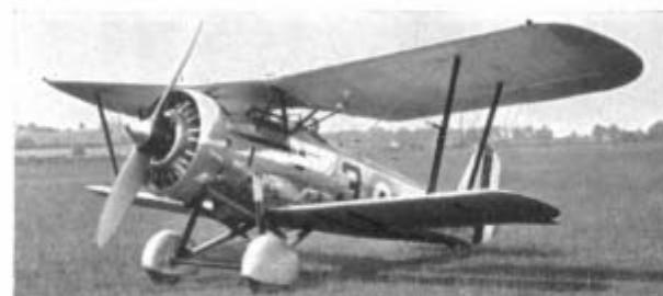
Above: Bulldog IIIA, R-5, c/n 7560, prototype. Built as private venture and first flown 17th September 1931. Mercury IVA engine and spats. Below, top: R-5 with Mercury IVS.2 engine, June 1932. Bottom: R-5 without cowling and spats and with Mercury IVS engine.
