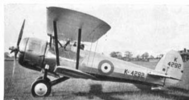
Left: R-7, K4292, with Perseus long-chord cowling, two-blade propeller and tail wheel. Right: K4292 with Mercury VIS-2 in long-chord cowling and Hamilton three-blade, variable-pitch propeller, July 1934.
