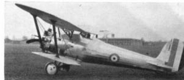
Bulldog II prototype with lengthened fuselage, experimental engine helmets and head-rest.
