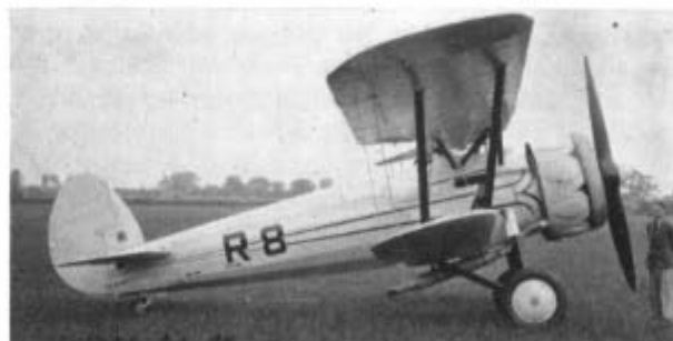
The second Bulldog IVA, R-8, c/n 7808. Registered G-ACJN and built to test Mercury VIS.2 engine. Later fitted with this engine, but first used for testing Perseus 1A. Seen here painted ready for the 1934 SBAC Show.
