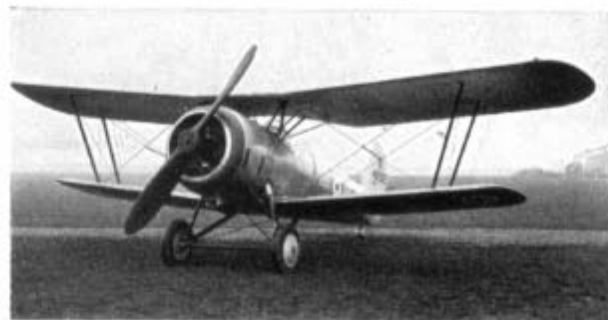
Left: R-7, K4292, with Perseus long-chord cowling, two-blade propeller and tail wheel. Right: K4292 with Mercury VIS-2 in long-chord cowling and Hamilton three-blade, variable-pitch propeller, July 1934.
