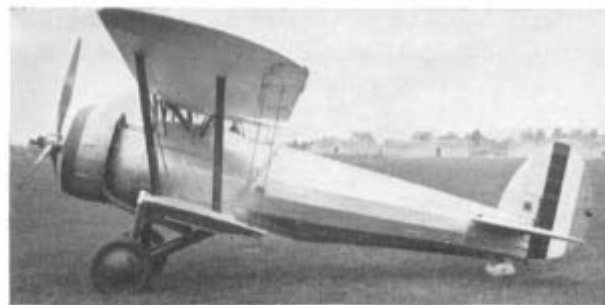
R-7, in its intermediate form with Mercury VIS.2 engine, short-chord cowling and Hamilton variable-pitch, three-blade propeller. Note twin aileron wires instead of strut.
