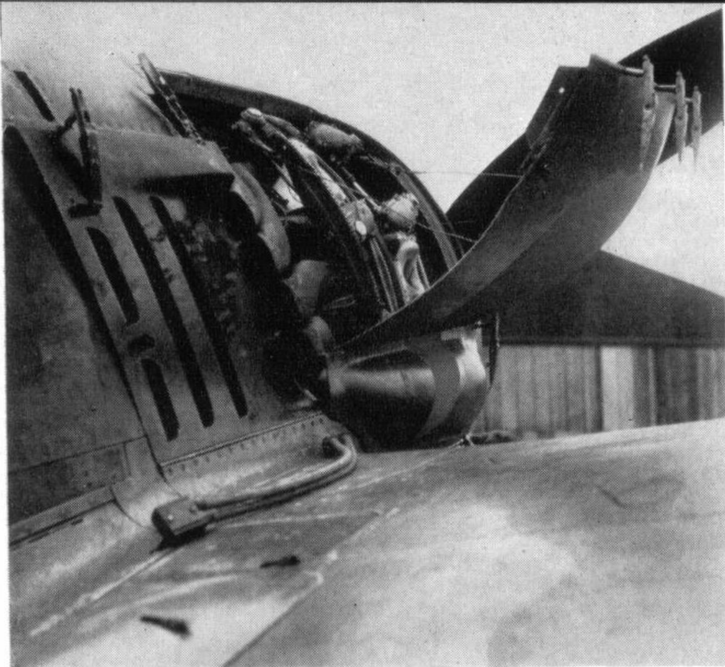
Exhaust detail of Fw 190A-3.
