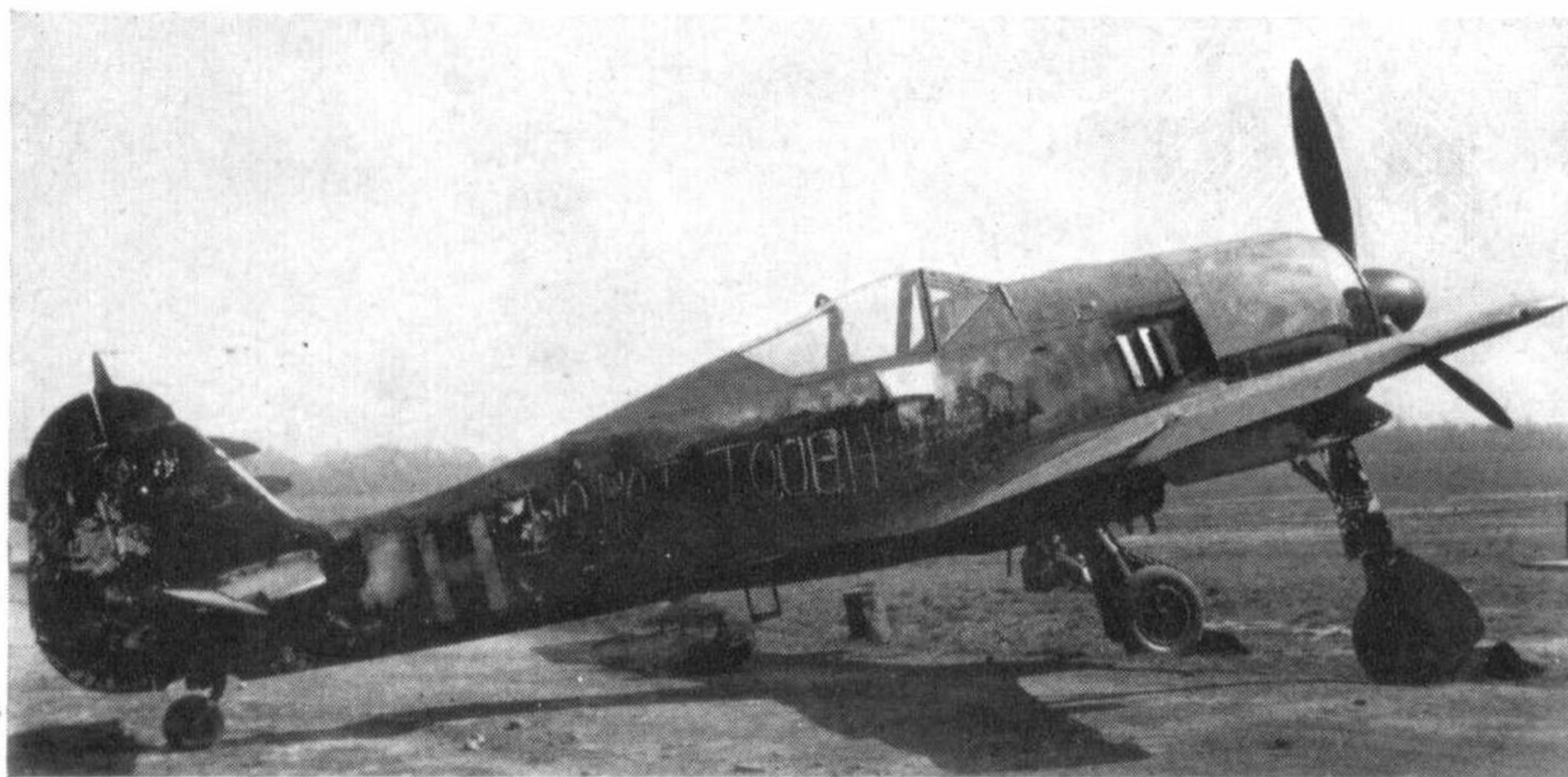
An Fw 190A-4/U8 of SKG 10 which landed at R.A.F. West Malling on the night of 16th July 1943. A matt-black temporary finish was applied to the aircraft for night intruder sorties.
