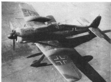
Two views of the Fw 190A-4/R5, with overwing tank experimental installation.
