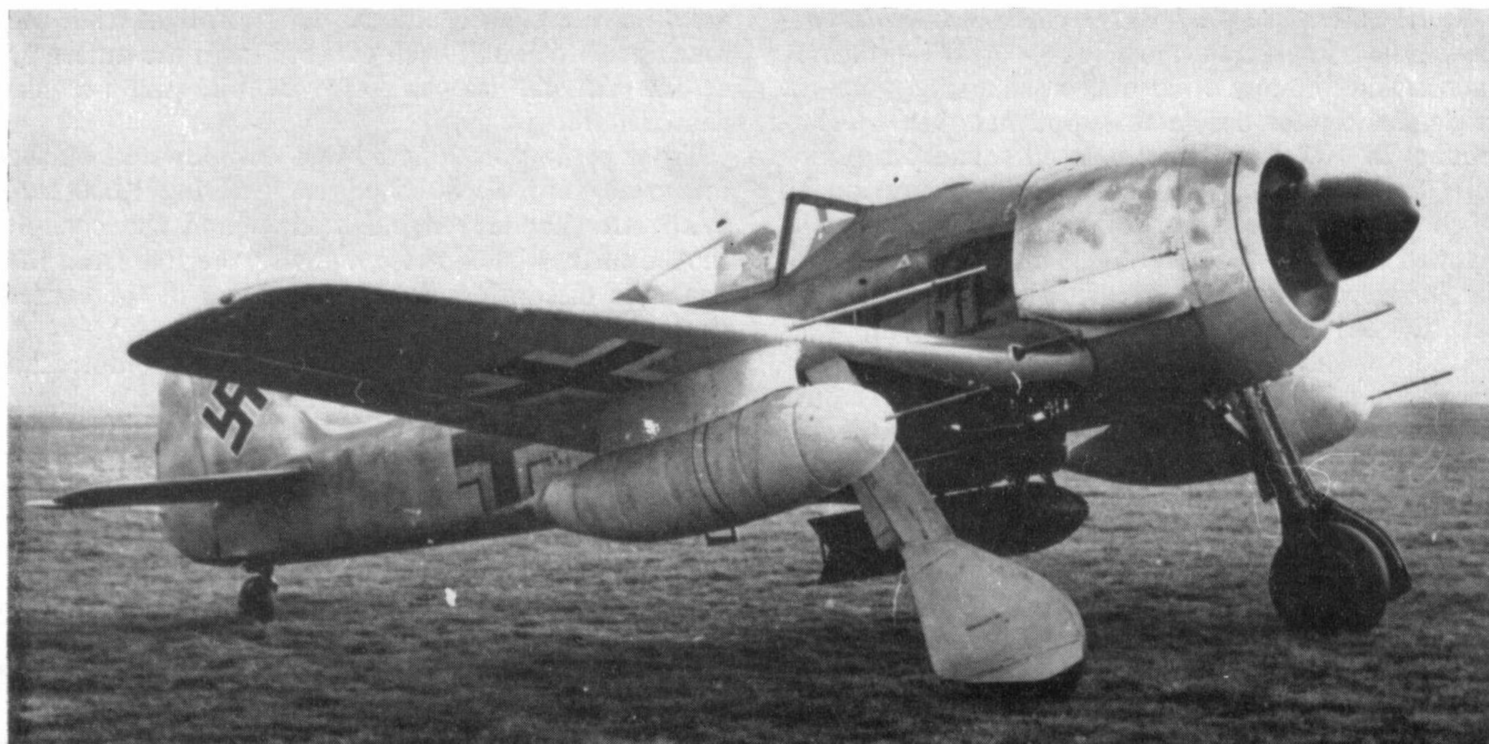
The A-4/U8 fighter-bomber with underwing tanks fitted.
