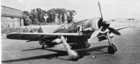
The A-5/U3 Trop sub-variant with bomb-load in place.
