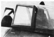
Left: Detail view of the A-3/U4 camera fairing. Right: Heavily armoured modification to an Fw 190A cockpit canopy.
