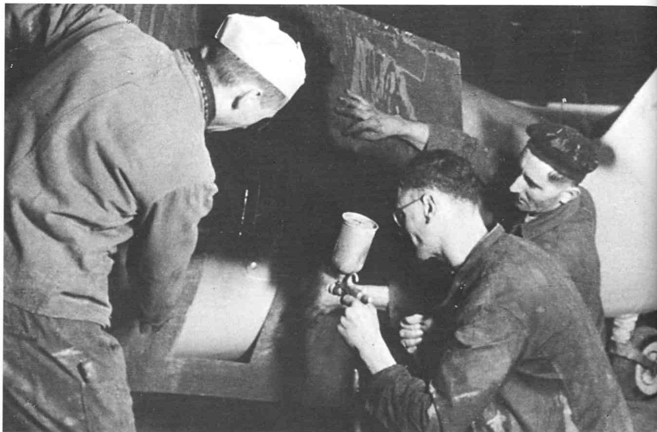
Above: The responsibility for painting new aircraft belonged to the each ground crew. These 'black men' are using a large stencil to spray the black-and-white Balkenkreuz over this aircraft's overall bright blue surface.
