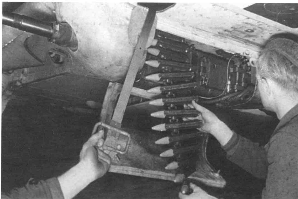
Left: A few Bf 109G-6/U4s and some K-4/U4s were rebuilt to allow for the installation of two bulges, each housing a heavy MK 108 gun. The belt shown being held by a member of the ground-crew was used to pull the ammunition into its storage space within both wing sections. Note the massive grenade heads on each shell. The explosive power of just one or two of these shells was believed sufficient to destroy a heavy bomber.
