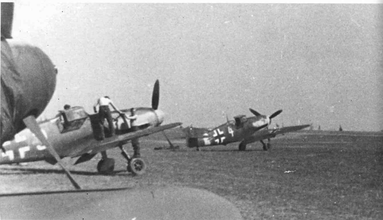
Below: In summer 1942 II/JG 51 was equipped with Bf 109F-2 and F-4 piston-engined fighters. To avoid being caught unprepared by Russian low-level attacks, many German units set up light anti-aircraft weapons or MG 34 machine-guns near accommodation areas.
