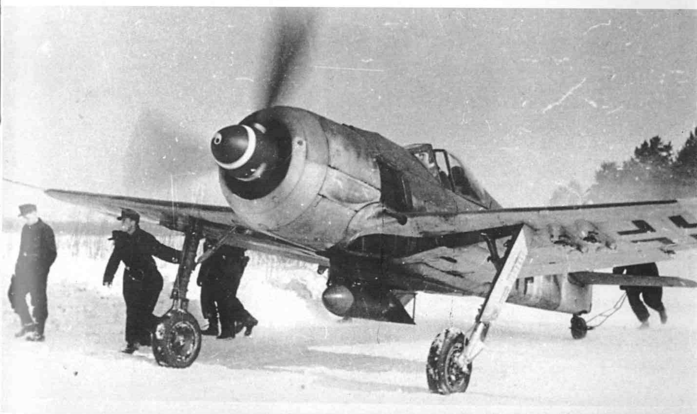
Bottom right: During winter 1944-5 this FW 190F-8 taxis to its take-off position with the help of its ground-crew, who are trying to control the aircraft's direction on the slippery surface. The fighter-bomber is loaded with one large SC 250 or SC 500 fragmentation bomb. It could also carry four SC 50s, SD 50s or SD 71s on the wings (note racks).
