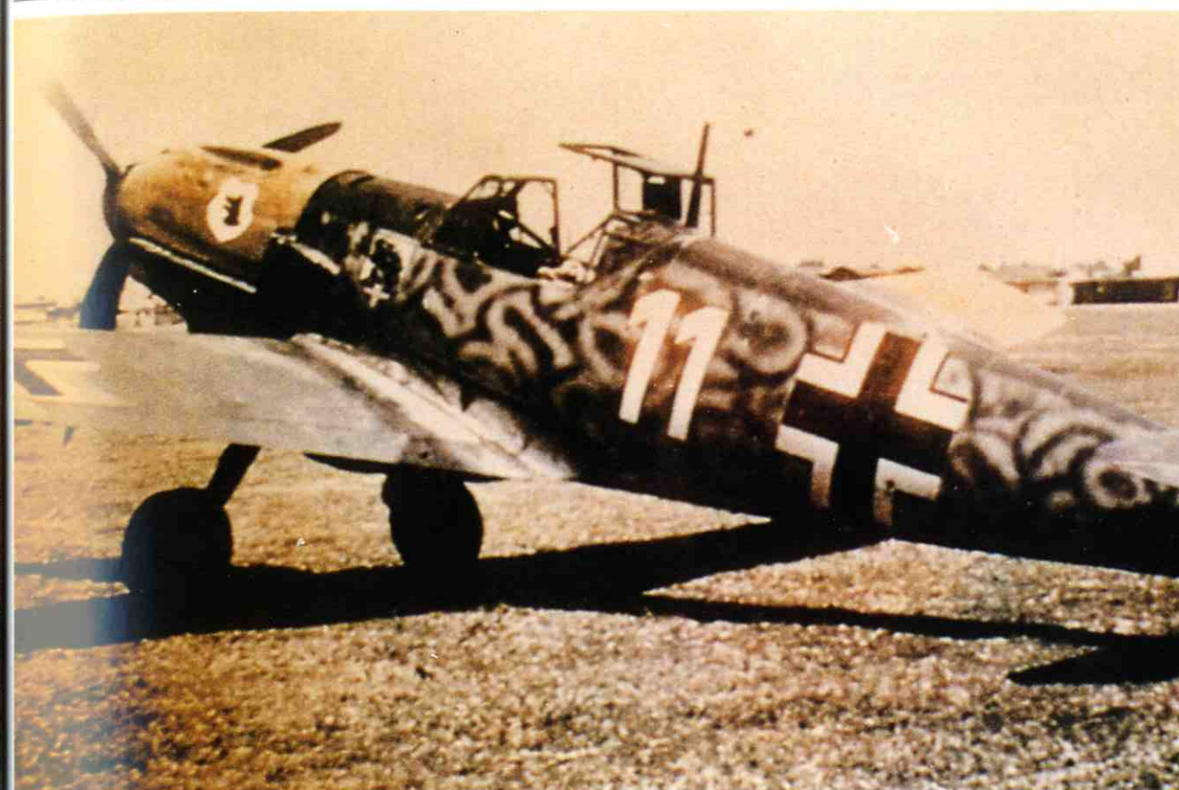
Above: A Bf 109 E 'White 11' of II/JG 54, handed over to a training unit after the first Bf 109F fighters had arrived in the Russian theatre. Because the ground at forward airfields was a different colour, the aircraft's earlier camouflage has been painted over with a darker mottled pattern to give it a better chance of surviving low level attacks by Red Army aircraft.
