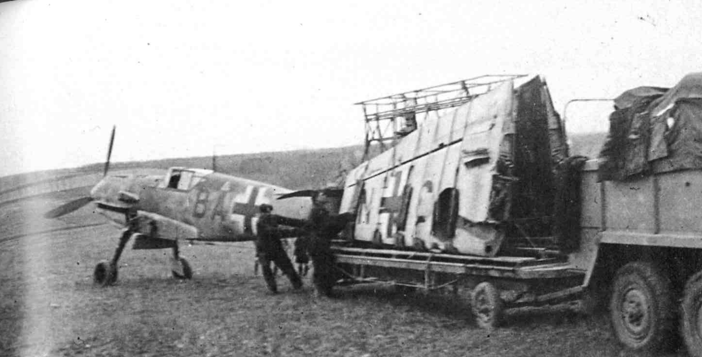
Above: During the opening stages of the invasion of Russia several Bf 109Es were lost due to enemy action. Additional losses resulted from technical problems or pilot error behind enemy lines. Aircraft which crashed on their own side of the front line were retrieved by specially-equipped recovery units.
