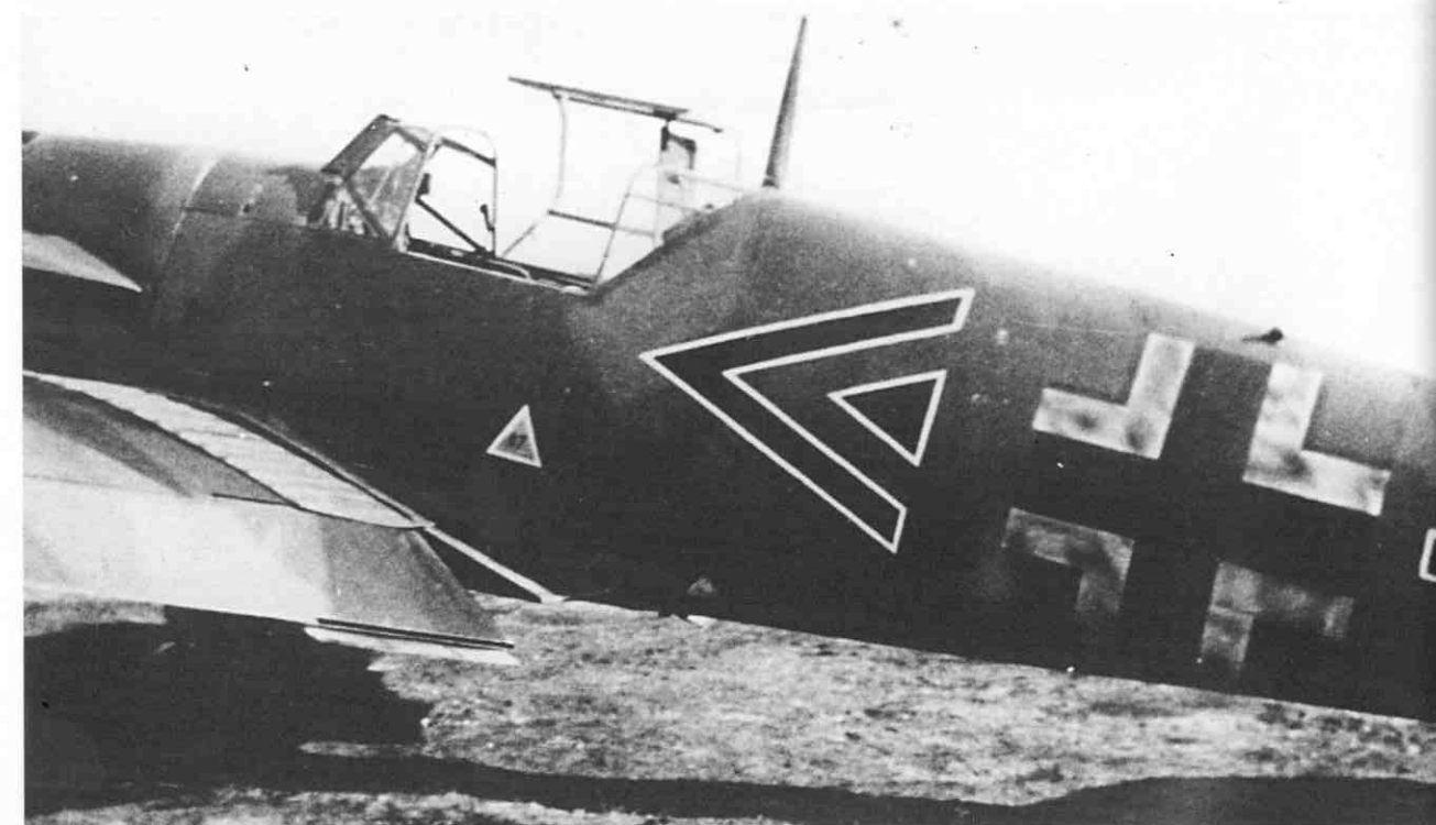
Above: In 1941, the Kommodore of JG 52, Major Hans Trübenbach, flew one of the new Bf 109F-4s (s/n 7090), which was manufactured by Wiener-Neustädter Flugzeugwerke (WNF) near Vienna in June 1941. Trübenbach's aircraft was photographed on October 1941 at Tiraspol. On the left side of its fuselage the triangle specifying 87 octane fuel for the aircraft's DB 603 E engine can be clearly seen.
