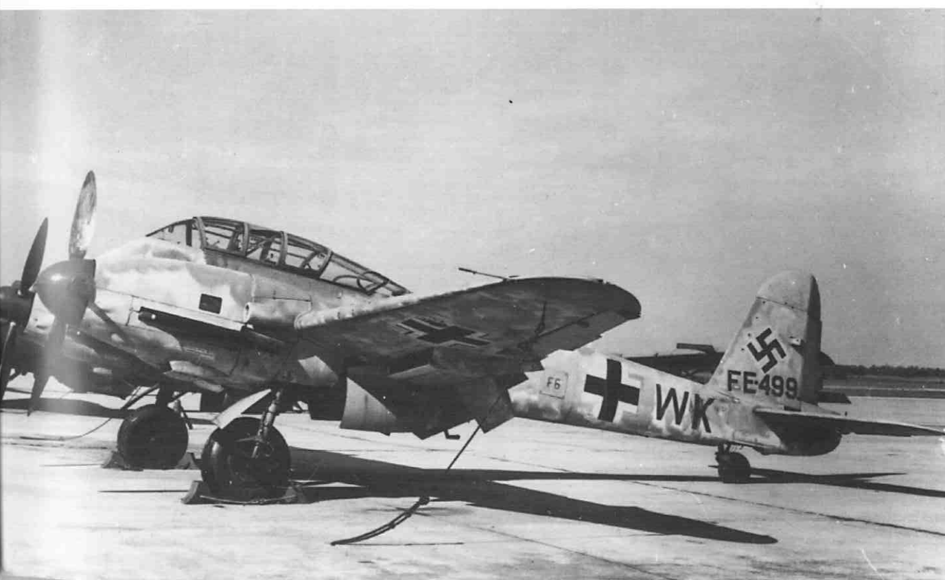
Above: When it became obvious that the Messerschmitt Bf 210 was a failure, the next step was the Me 310, with a pressurised cockpit and more powerful engines. This was subsequently abandoned in favour of the Me 410 Hornisse . The Hornisse was essentially the Bf 210 with DB 603A engines. Featured here is the Me 410A-1 fast bomber, with rearward-facing guns in remotely-controlled barbettes.
