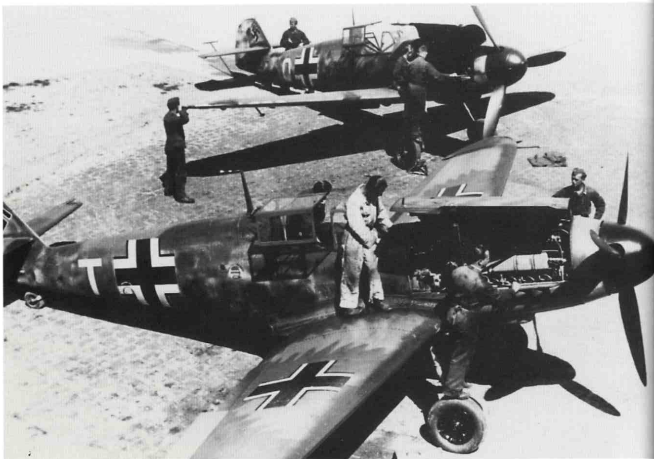
Below: By the beginning of 1943, the Messerschmitt Bf 109G series had almost entirely supplanted earlier models. With wheels and flaps down, it had to be flown at full throttle even when landing. These are two Bf 109G-4s of an unidentified Reich home defence unit.
