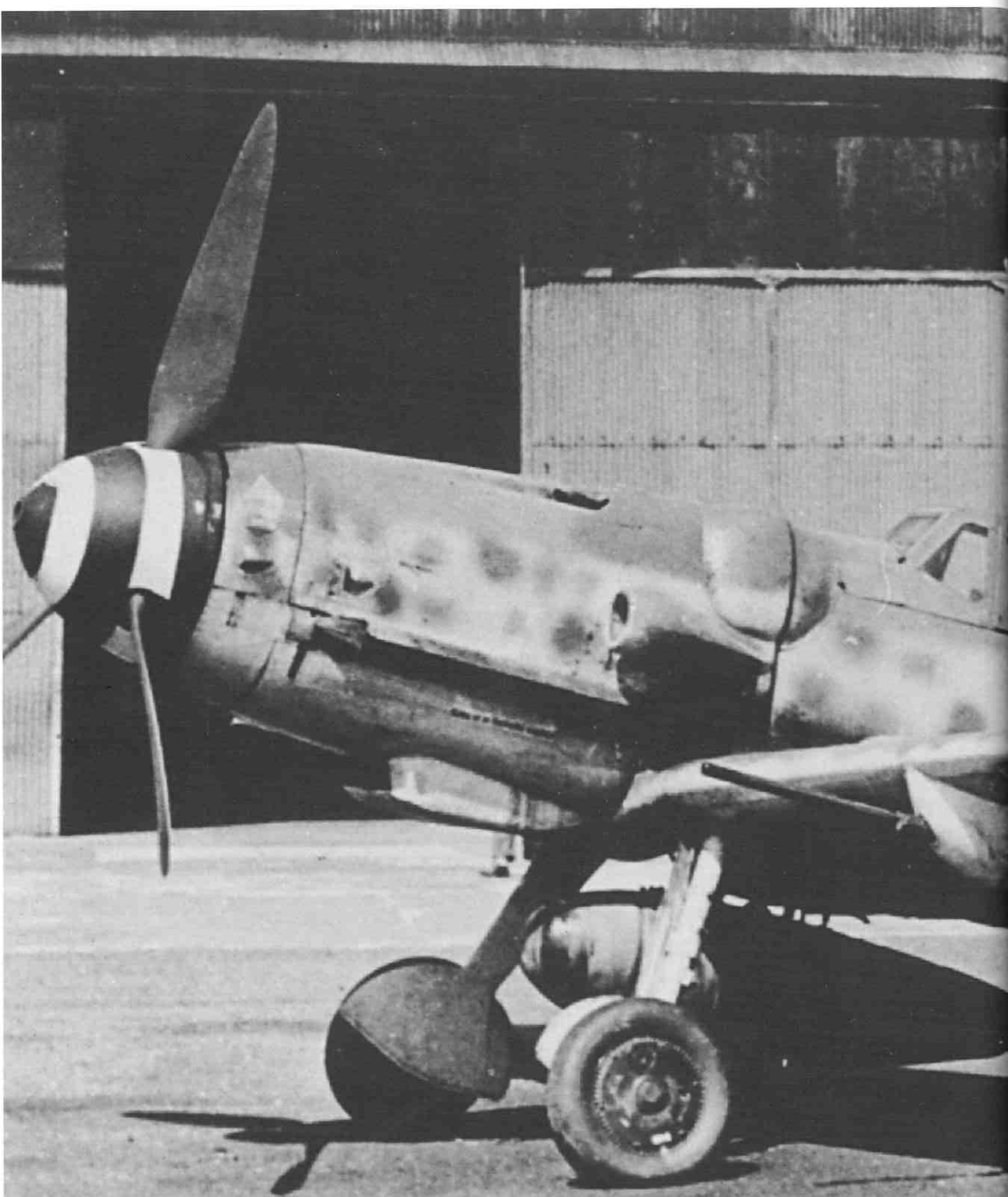
The most numerically important of the Messerschmitt Bf 109G series was the G-6. It was armed with a single 30 mm MK 108 cannon firing through the spinner, and two 13 mm heavy machine guns mounted above the engine. Bulges covering the machine gun breeches and ammunition feeds which gave the Gustav its nickname of Beulen (bumps); one is visible just ahead of the cockpit. It also boasted two 20 mm cannon in underwing pods. This example, formerly White 14 of JG 1, landed at Manston in the early hours of 21 July 1944.
