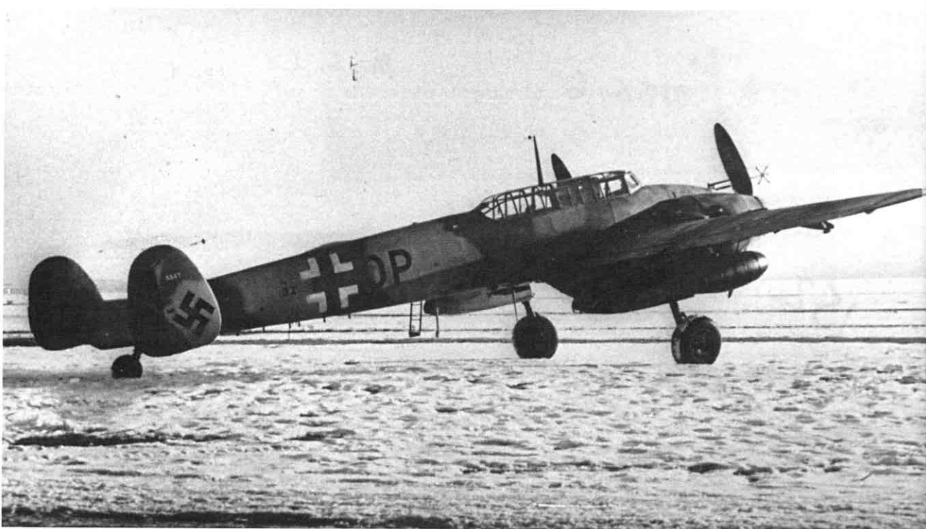
Above: This Bf 110G-4 carries a modified day fighter camouflage and still has the small fins of a Bf 110F aircraft. It belonged to 7 Staffel of NJG 5 (2Z+). Being engaged in long-range defensive missions, this aircraft is provided with two 300-litre drop tanks. After commissioning, 7/NJG 5 saw operational service until the end of the war under the command of Hauptmann Leuchs and Hauptmann Helmuth Schulte.
