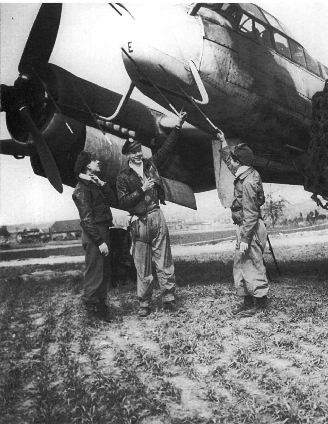
Early in 1945 the first Ju 88G-6s were captured by Allied forces in northern Germany. These USAAF officer are examining the AI radar installation of this G-6. Note the open entrance hatch and the two MG 151/20 weapons fitted in the weapon bulge together with two further MK 108 guns.
