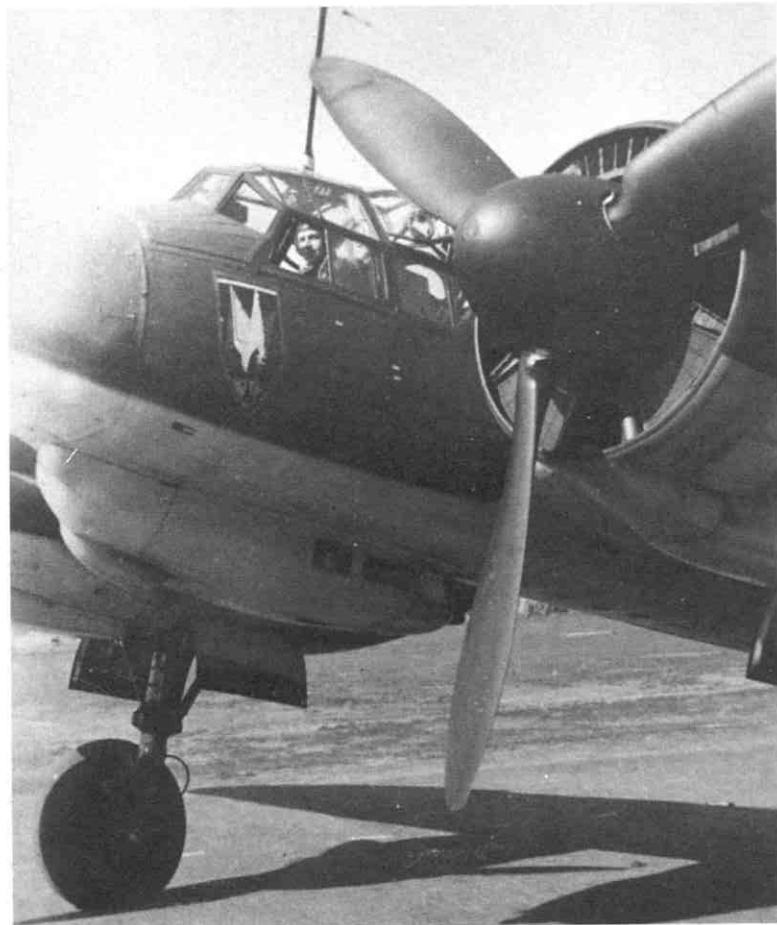
Left: The Ju 88C-4, which was in service from 1941 to late summer 1944, was powered by either two Jumo 211 B or two C piston engines. Its forward armament consisted of five MG 15s and one 20 mm MG FF aircraft cannon. Many C-types were called Mischausführungen because they were rebuilt bomber aircraft or modified heavy fighters.
