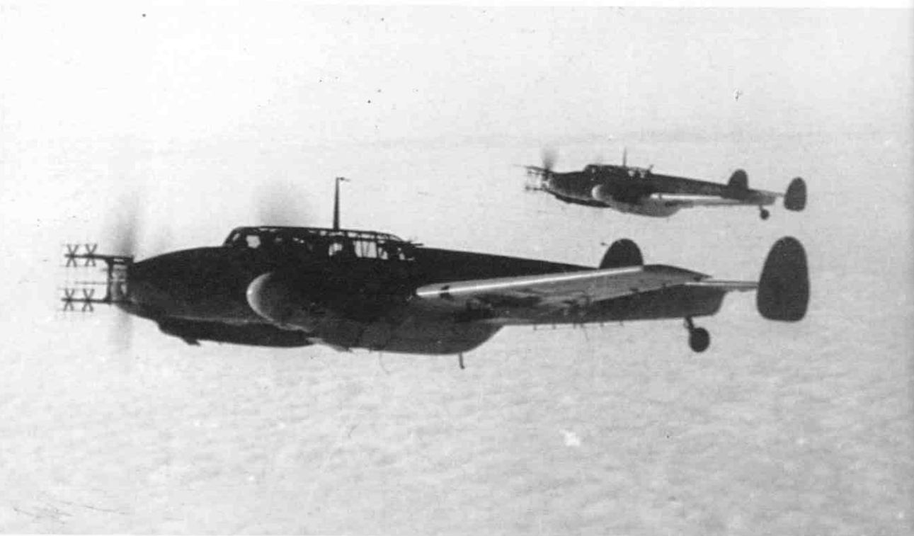
Above: This Bf 110G-4 carries a modified day fighter camouflage and still has the small fins of a Bf 110F aircraft. It belonged to 7 Staffel of NJG 5 (2Z+). Being engaged in long-range defensive missions, this aircraft is provided with two 300-litre drop tanks. After commissioning, 7/NJG 5 saw operational service until the end of the war under the command of Hauptmann Leuchs and Hauptmann Helmuth Schulte.
