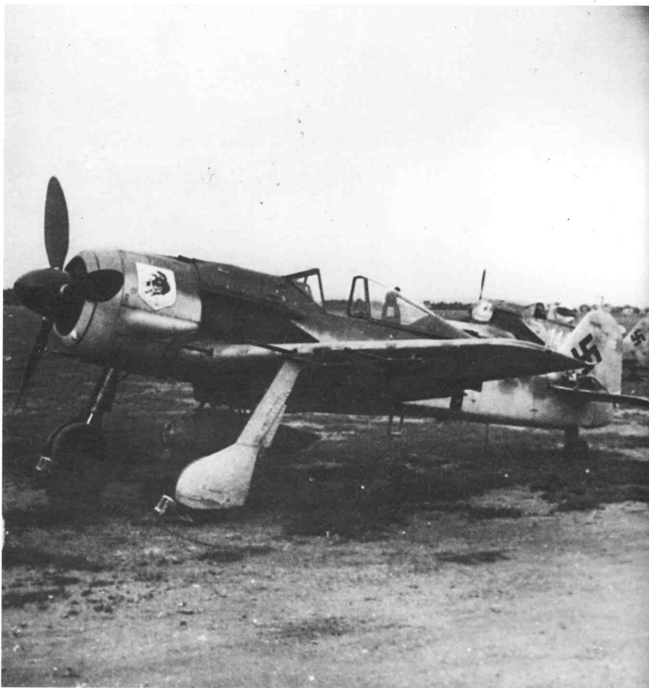
Only a handful of FW 190A-6s were flown with a FuG 217 'Neptun' radar installed. This aircraft, fitted with four antennae, was flown by Oberfeldwebel Migge, serving with 1 Staffel of NJGr 10 at Werneuchen. Besides this formation, many single-engine nightfighters were concentrated in the hands of NJG 11's pilots, one of whom was Leutnant Kurt Welter, who became the commanding officer of the Me 262-equipped 10/NJG 11.
