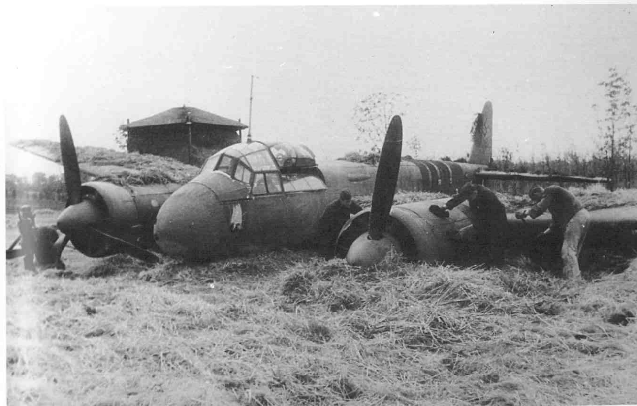
Below: This crashed Ju 88C has been well camouflaged by its ground crew to provide protection against fighter-bomber attack. The aircraft was one of the Mischtypen or 'mixed types', a cross between the Ju 88C-4 and C-6 arrived at by using assorted spare parts. Many late Luftwaffe combat aircraft were pieced together from parts belonging to different series and were not listed in any official handbook.
