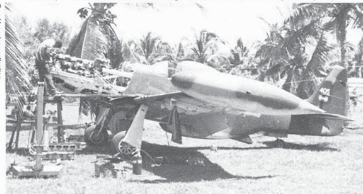
Field maintenance on "Mustangs" was commonplace in Salvador during the 1969 hostilities. FAS 405 undergoes major powerplant maintenance. This view provides good detail of the left wingtip fuel tank and the rather primitive working conditions.
