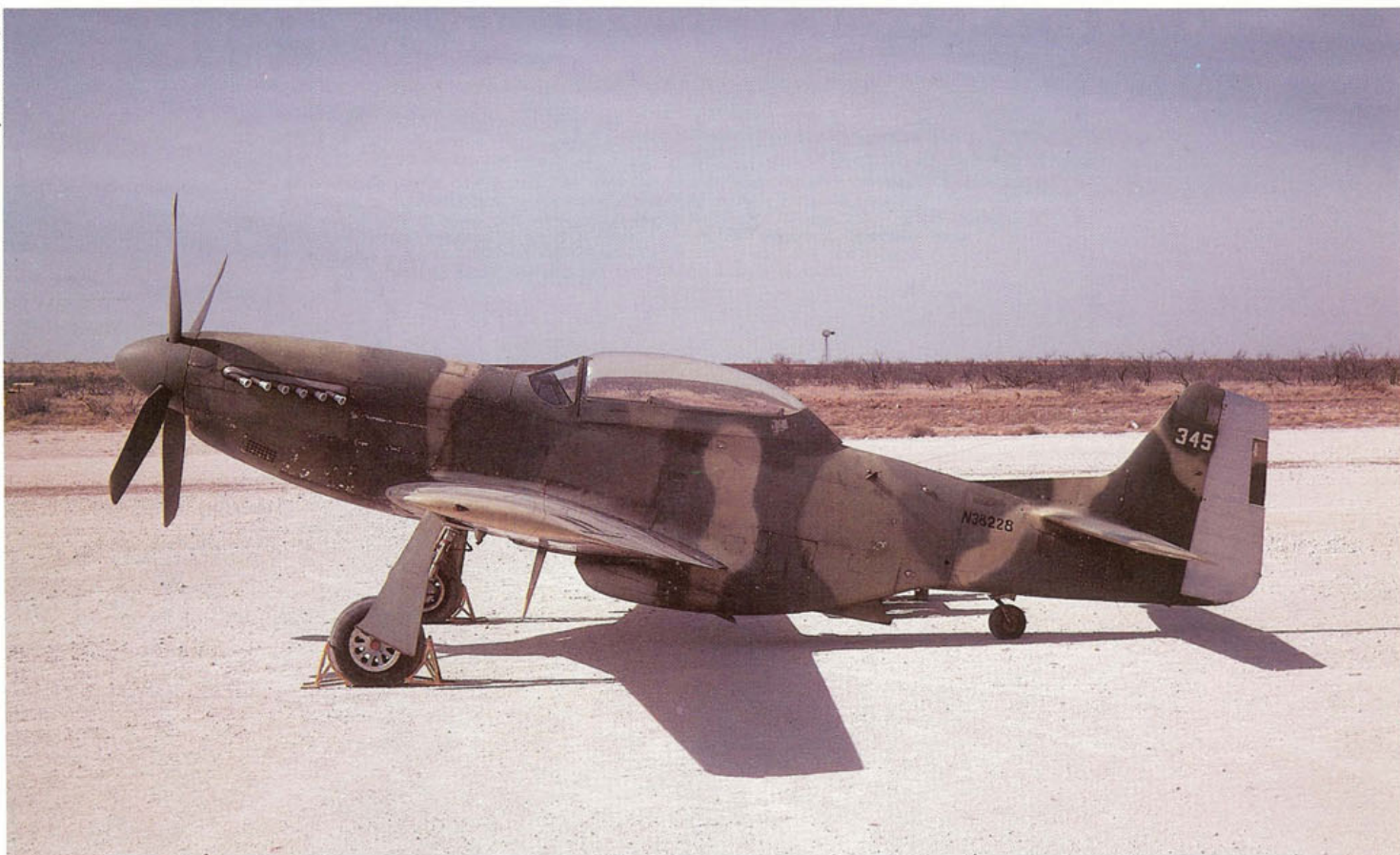
Ex-Guatemalan Air Force TF-51D, FAG 345, civil-registered N-38228, shortly after its return to the U.S. under the auspices of Connie Edwards. This two-seat aircraft has the extended canopy and internal modifications required for the training role. The primed, but unpainted rudder is the only surface on the aircraft not still in the original FAG camouflage. Noteworthy are the plastic cups used to keep condensation out of the cylinders.
