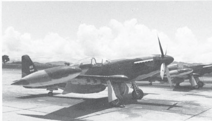
Two Cavalier "Mustang II's" of the Salvadoran Air Force, FAS 401 and FAS 402, respectively, shortly after their delivery to El Salvador. These aircraft were equipped with numerous improvements including tip tanks and an extended vertical fin.
