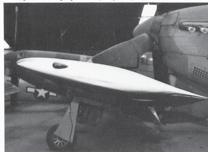
The "Mustang's" airfoil section was of the laminar flow type. It was developed to help alleviate the effects of compression while flying at near-sonic velocities. By delaying shock-wave development, performance could be considerably improved.
