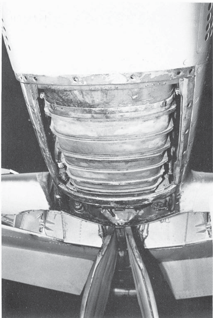
The duct intermediate section is located underneath the engine and serves, with the rest of the duct, to funnel air from an intake located below and just aft of the propeller spinner to the engine carburetor.
