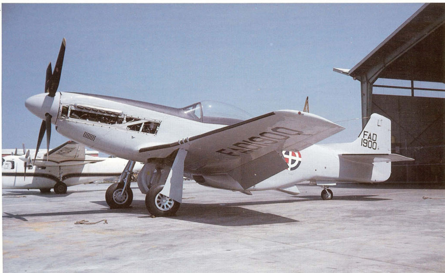
Dominican Air Force F-51D, FAD 1900, following modification accomplished at the Trans-Florida Aviation facility at Sarasota, Florida, during February and March, 1965. The FAD insignia is visible on the fuselage side. Discernible under the left wing is the FAD 1900 identification marking. Noteworthy, too, is the black-painted leading edge. The light gray scheme shown would eventually give way to a more contemporary over-all green and tan camouflage, with several other schemes applied in the interim.
