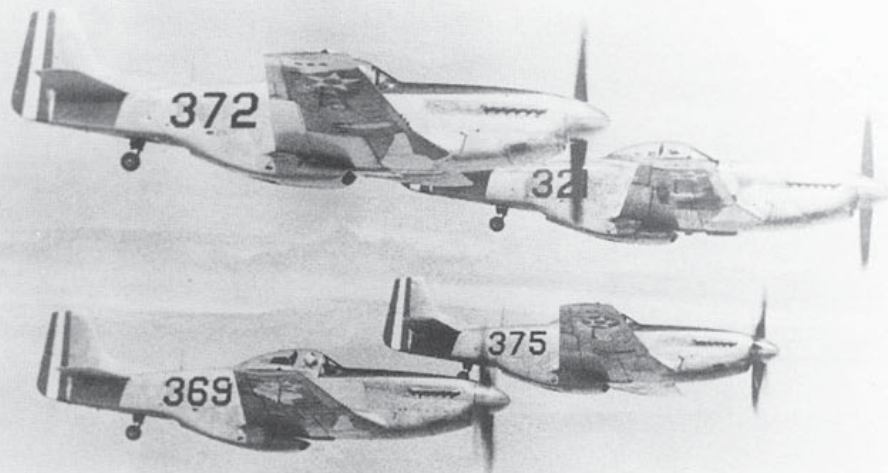
A quartet of Guatemalan Air Force F-51D's in formation flight. Still visible under the wings are the outlines of the USAF insignia. Extended tailwheel was the end result of a long-standing F-51 maintenance anomaly that was more easily rectified by leaving the gear down than by solving the problem.
