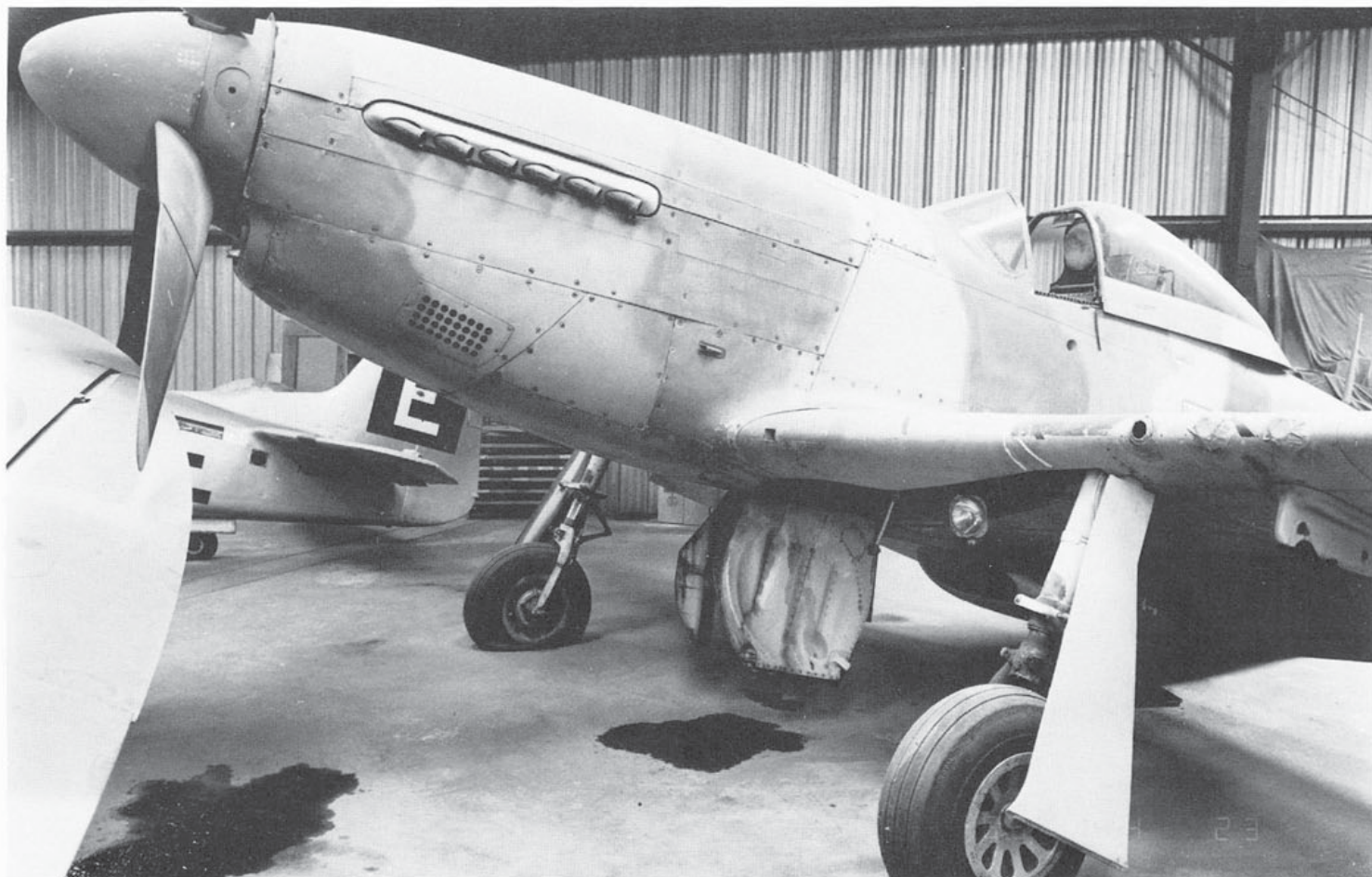
Barely visible in this view is a round, flat metal plate mounted just behind the propeller spinner. This plate was found necessary in order to prevent propeller seal oil leak accumulations on the aircraft windscreen. The wind blast forced the oil onto the plate which caused oil spray to accumulate there. In this way, the windscreen was spared, thus allowing the pilot a good forward view. This minor modification is not often applied to civil "Mustangs" seen flying today.
