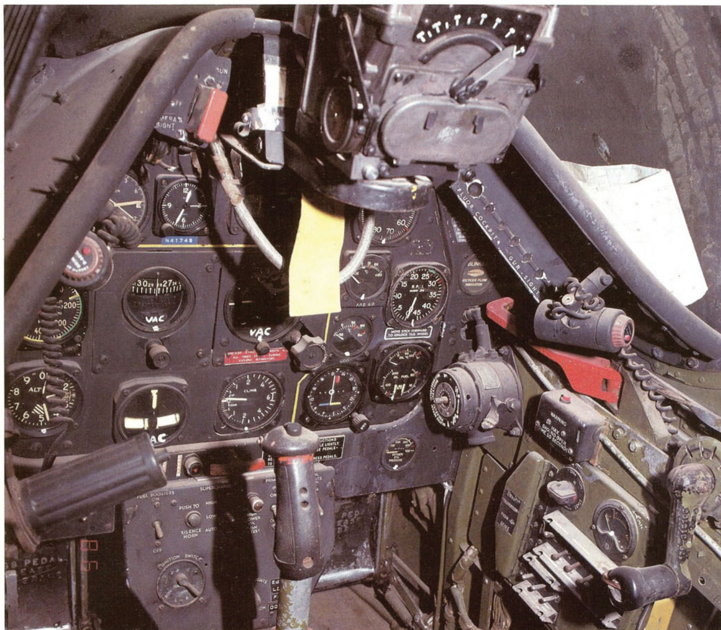
Forward instrument panel of an ex-Guatemalan F-51D, civil-registered, N-41749. The panel is stock for the type in FAG service, with full analogue instrumentation and a conventional panel-mounted gunsight. Visible to the left is the throttle quadrant. At right center is the oxygen regulator, sans hose. The control stick also is stock for type, with a mic switch on top and a weapon switch on the grip front (not visible).
