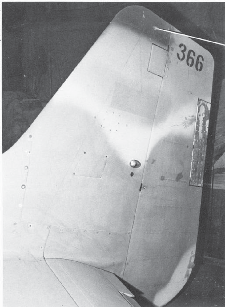
Though the "Mustang's" vertical fin assembly was of all metal construction, the hinged rudder assembly remained fabric covered. The rudder, like the elevators, was equipped with a trim tab and a single large mass balance of lead.
