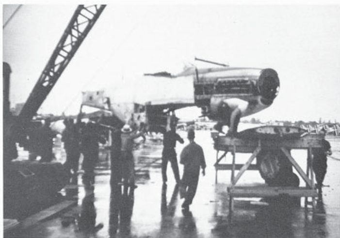
Following their arrival during 1952, the dismembered ex-Royal Swedish Air Force "Mustang's" were reassembled at Ciudad Trujillo, Salvador, using indigenous labor and the assistance of Swedish maintenance personnel.
