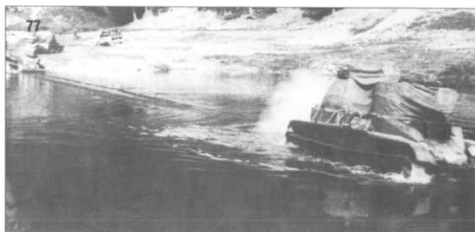
77,78. Испытания опытного танка подводного буксирования БТ-5ПБ. Август, 1934 г. The evaluations of the BT-5PB — the tank capable of submerged water crossin being towed by another vehicle. August 1934.
