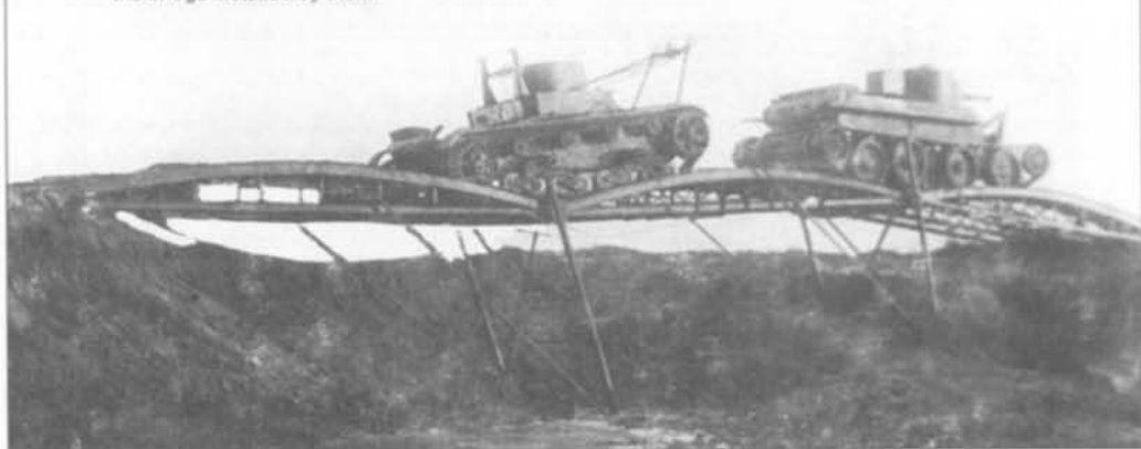
Преодоление саперными танками СТ-СБ (Т-26, БТ-5) оврага по наведенному ими мосту. Two engineering vehicles — the ST (based on the T-26), and the SB (based on the BT-5) cross the trench by the bridge installed by them.
